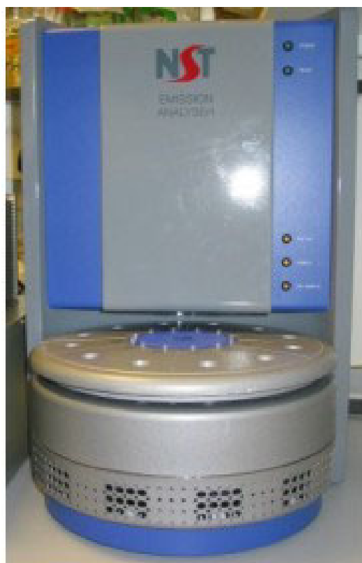
Plate 2.3 NST3220 Lab Emission Analyser with auto sampler carousel.
