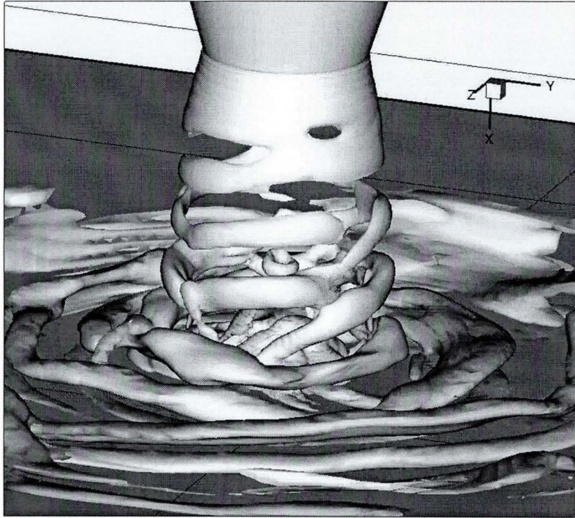
Figure 7.7: Instantaneous vortex structures around impingement point using iso-surface of Q
