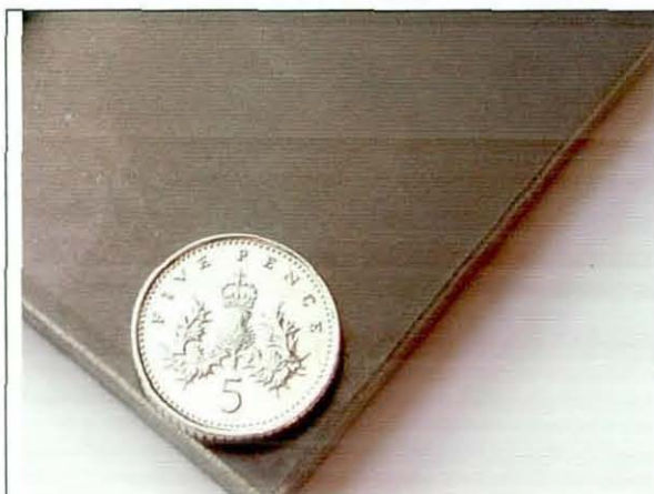
Figure 76. Macro photograph of Apticote 450 coating on nickel tooling. A five pence piece used for scale.
