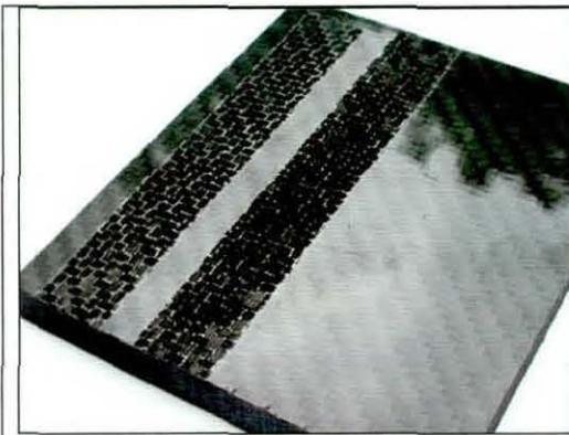
Figure 117. Photograph showing effect of TEA CO_2 laser on virgin composite tile. The resin rich gel coat has been striped by the laser to expose the carbon fibre matrix.
