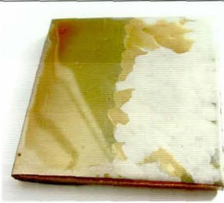
Figure 108. Photograph showing how bonded resin flakes away from Ni substrate after Nd:YAG laser cleaning.
