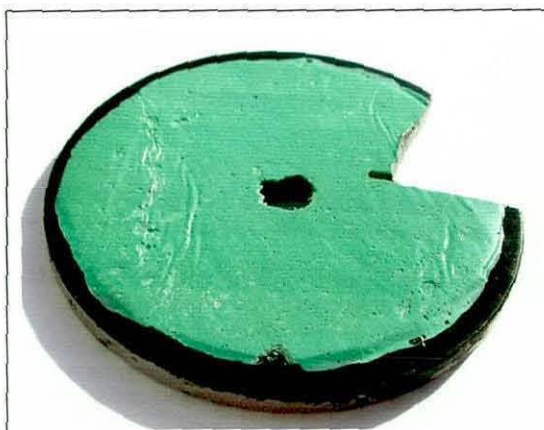
Figure 176. Photograph showing adhesion of FM300 resin to Xylar 2020 coating on steel blister test disc.
