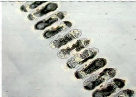
Figure 123. Close up macro-photograph showing effect of Nd:YAG laser used to clean resin bonded onto composite tile.
