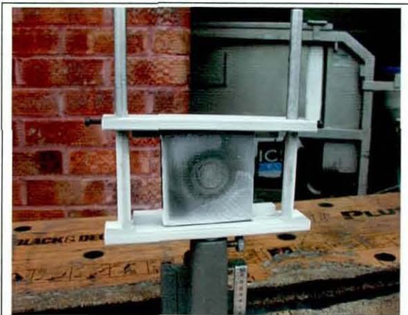
Figure 12. Dry ice blasted sample
