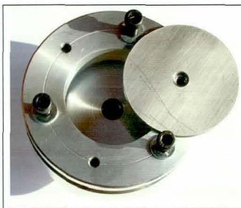
Figure 55. Blister test plate and cell
