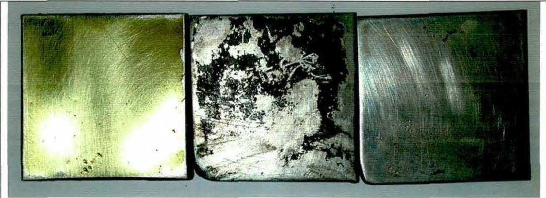
Figure 141. Treatment of resin coated nickel using the sodium hydride process
