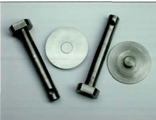
Figure 53. Axial butt test components. This figure shows two steel discs which each screw into the adjacent
