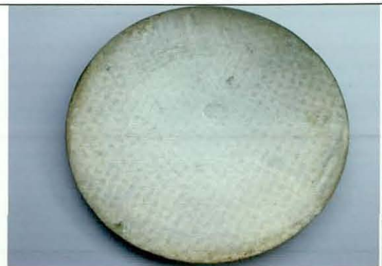
Figure 54. Used axial butt test disc. This disc was coated with Frekote and achieved 20 releases of prepreg cured
