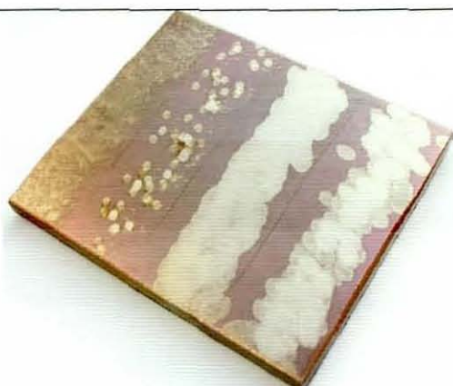
Figure 99. This figure depicts the partial cleaning of selected areas of contamination (similar to that shown in the previous figure) using a Nd:YAG laser at different cleaning fluences.
