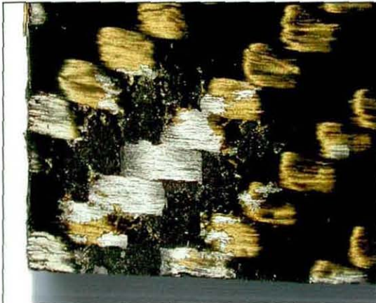
Figure 133. Dry ice blasted composite tile coated with resin (10 seconds treatment time at 5 bar).
