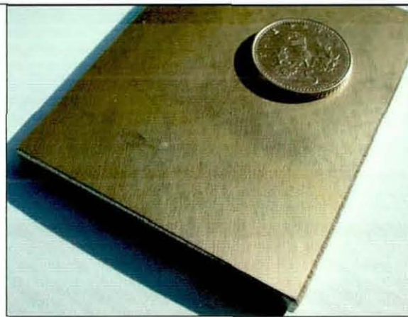
Figure 63. Macro-photograph of coupon of resinous contamination on nickel tooling ex-Bombardier.
