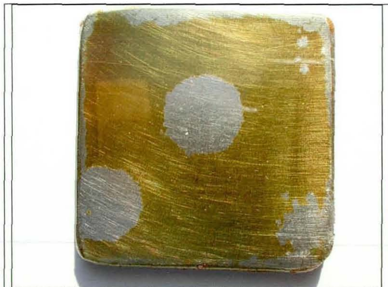
Figure 139. Resin coated nickel substrate dry ice blast treated for 5 seconds at 3,4,5,7 and 10 bar pressure.
