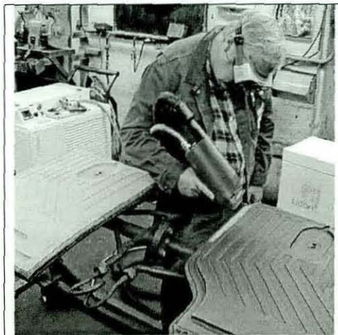
Figure 196. Commercial Nd:YAG laser cleaning system.
