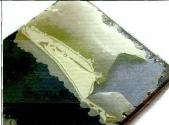
Figure 109. Photograph showing how bonded resin flakes away from steel substrate after Nd:YAG laser cleaning.
