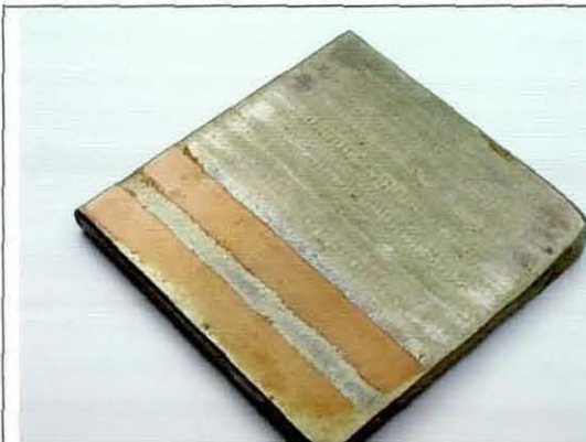
Figure 86. Effect of TEA CO 2 laser cleaning of epoxide resin from nickel tooling. Originally the epoxide resin covered the whole sample. The laser was then used to selectively remove the resin over most of the surface leaving two epoxide resin strips (depicted by the brown colouration) to contrast the areas cleaned against uncleaned areas.
