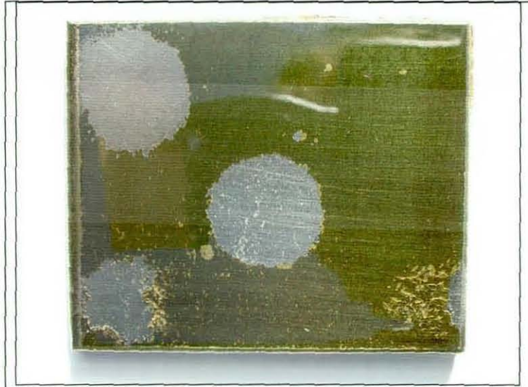
Figure 140 Resin coated steel dry ice blasted at 10 bar for 3,7,10 and 20 seconds.
