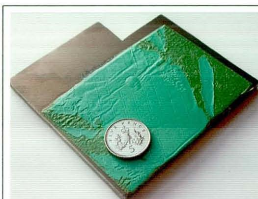
Figure 187. FM300 epoxide resin sheet cured onto Apticote 450 coated nickel substrate.
