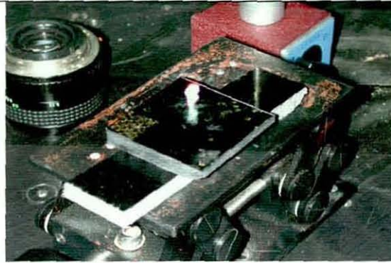
Figure 121. Photograph showing plasma effect when Nd:YAG laser focussed onto resin bonded to composite tile.
