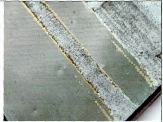
Figure 93. Macro-photograph at a slightly higher magnification of an area depicted in Figure 92. This more clearly contrasts cleaned and uncleaned areas (darker grey colouration with brown edges where the resin has been burnt during the laser cleaning).
