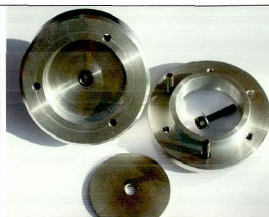
Figure 56. Blister test cell components
