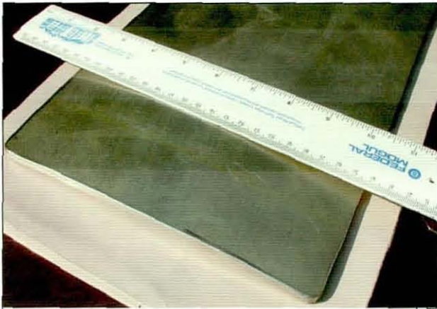
Figure 43. Example of contaminated nickel tooling
