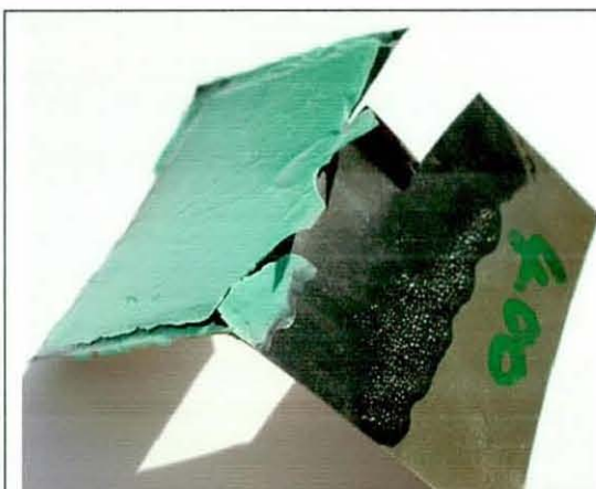
Figure 183. Xylan 8080 coating sintered onto stainless steel foil (black coating). FM300 resin (green) was then cured onto the Xylan coating.
