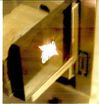
Figure 115. As Figure 114 showing a close up photograph of the laser focussed onto the composite tooling..
