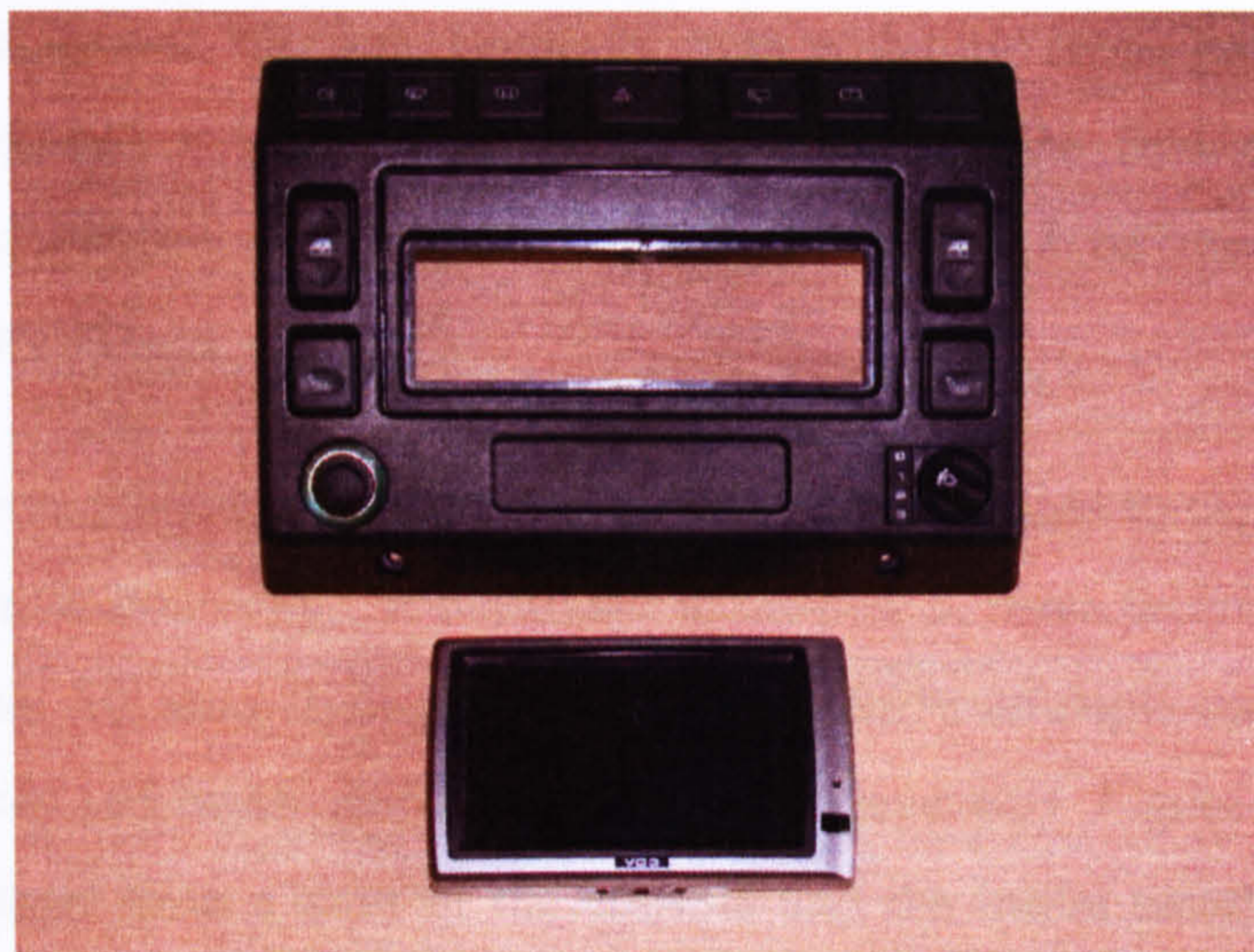
Figure 6.34: Current dashboard console and electronic navigation unit
