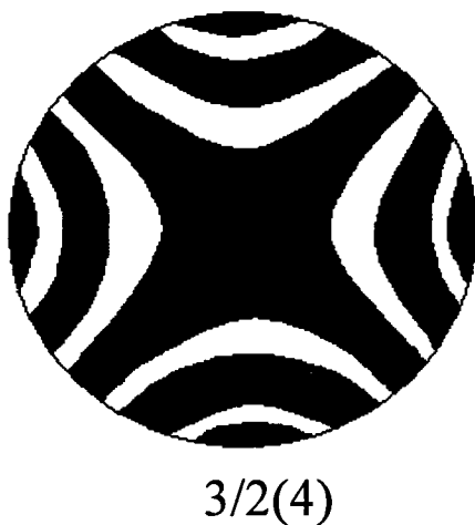
Figure 3.4. Fringe Pattern from an Astigmatic Surface where Non-Circular value is Greater than the Number of Complete Fringes Permitted
