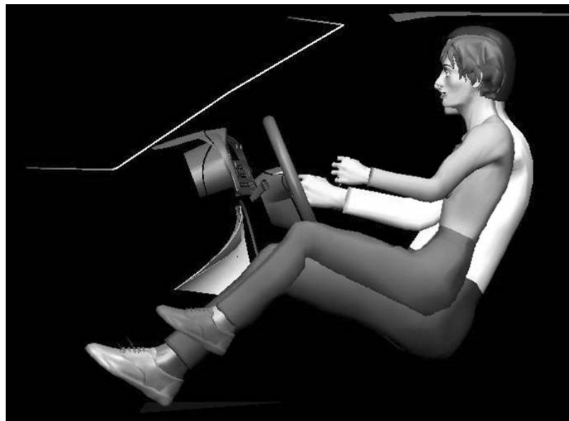
Figure 5.28. Fixed eye position. Tallest male and shortest female in A-CADRE shown.
