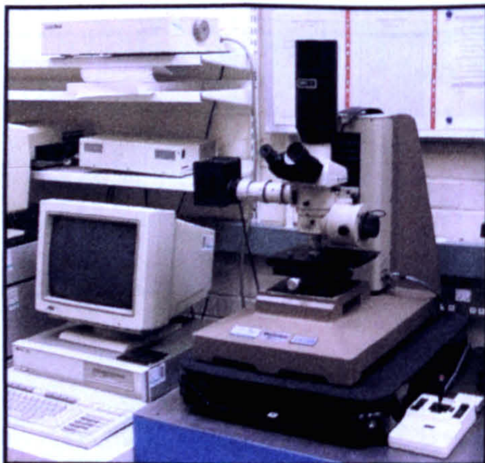
Figure 3.34 – Photograph of Wyko Topo-3D Surface Profiler
