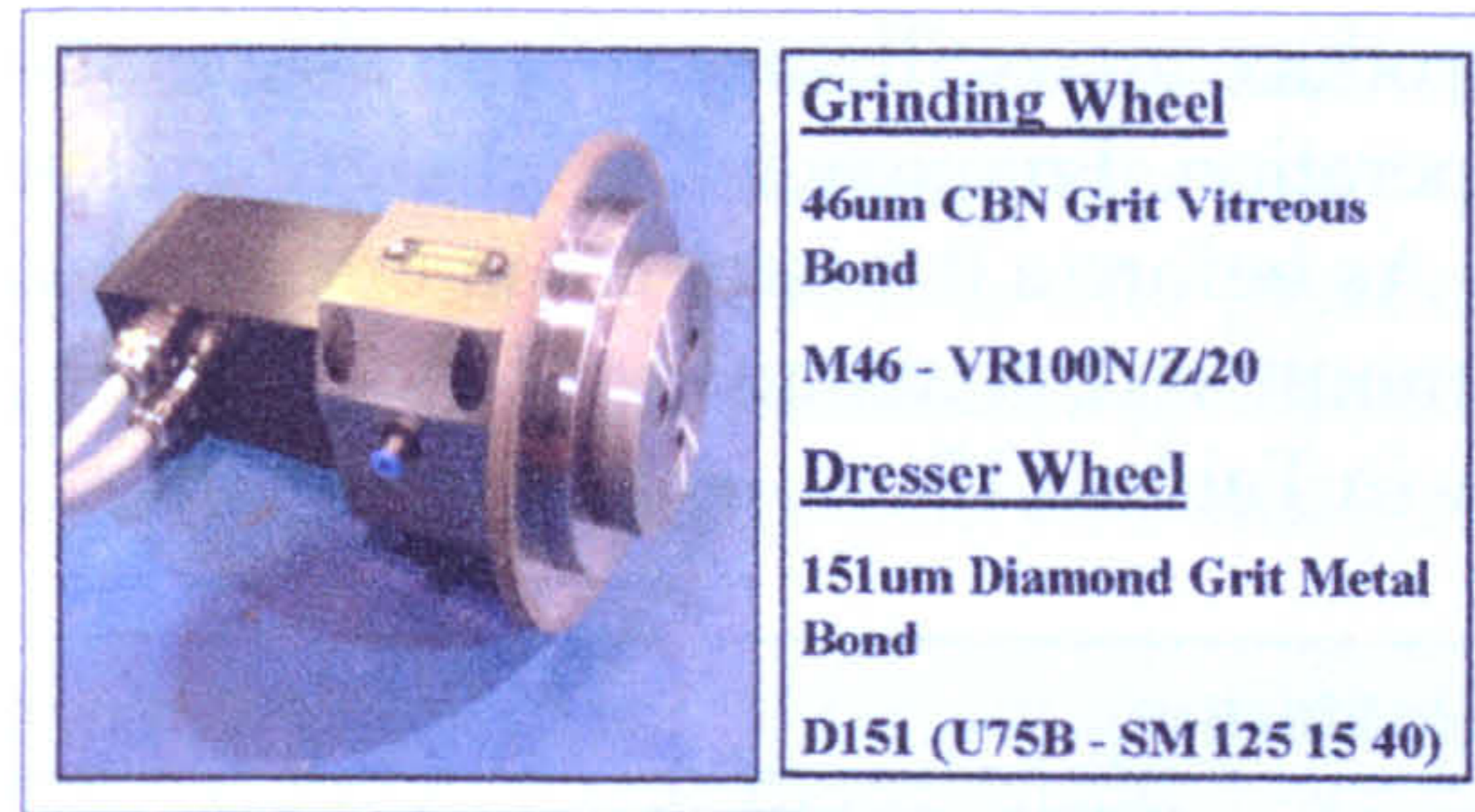
Figure 3.29 – Wendt Boart Dresser Spindle and Table of Wheel Specifications
