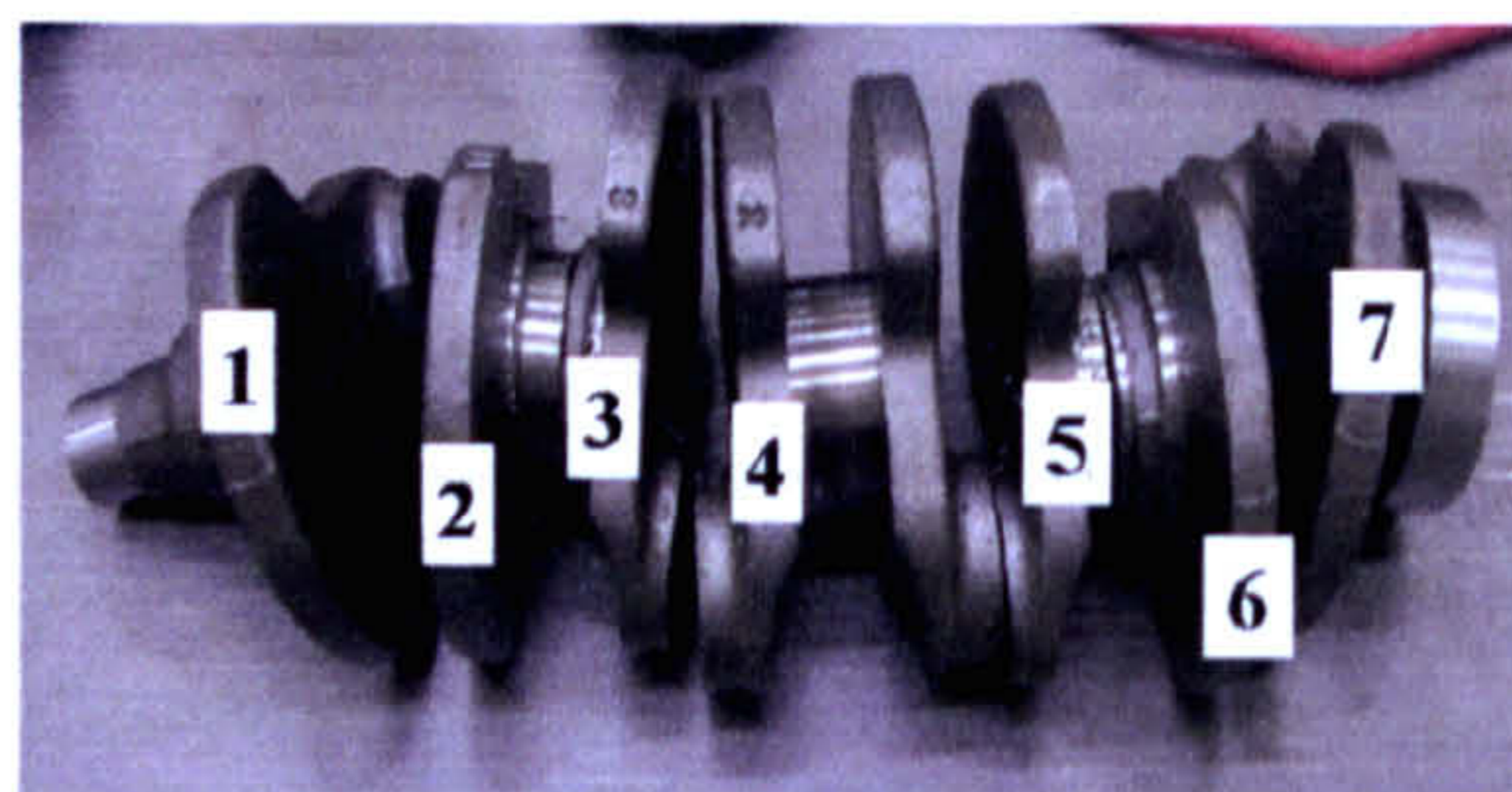
Figure 3.19 – Crankshaft Sectioned for Residual Stress Measurement
