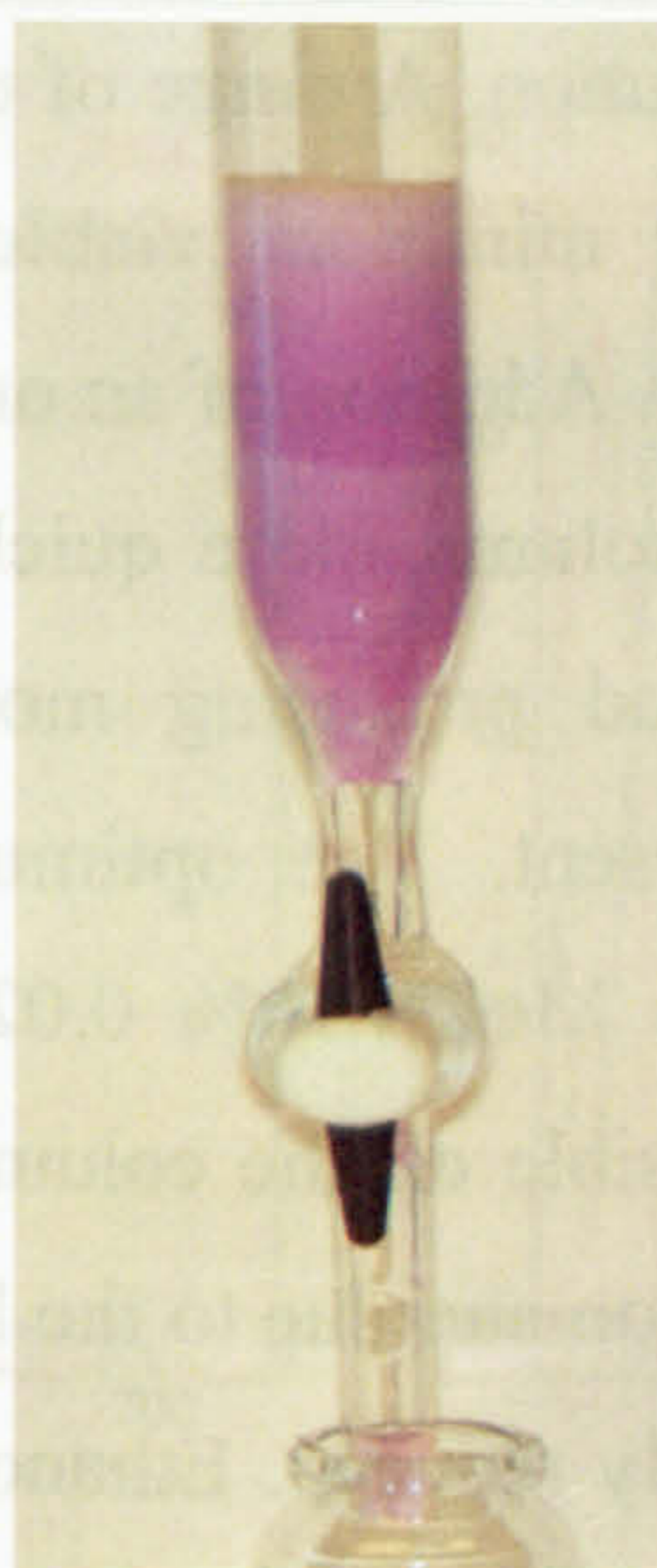
Figure 2.12 Cellulose column showing enantiomeric separation of parent compound.
