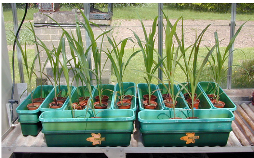
Plate 2.3. Pots arranged in plastic trays for leachate collection.
