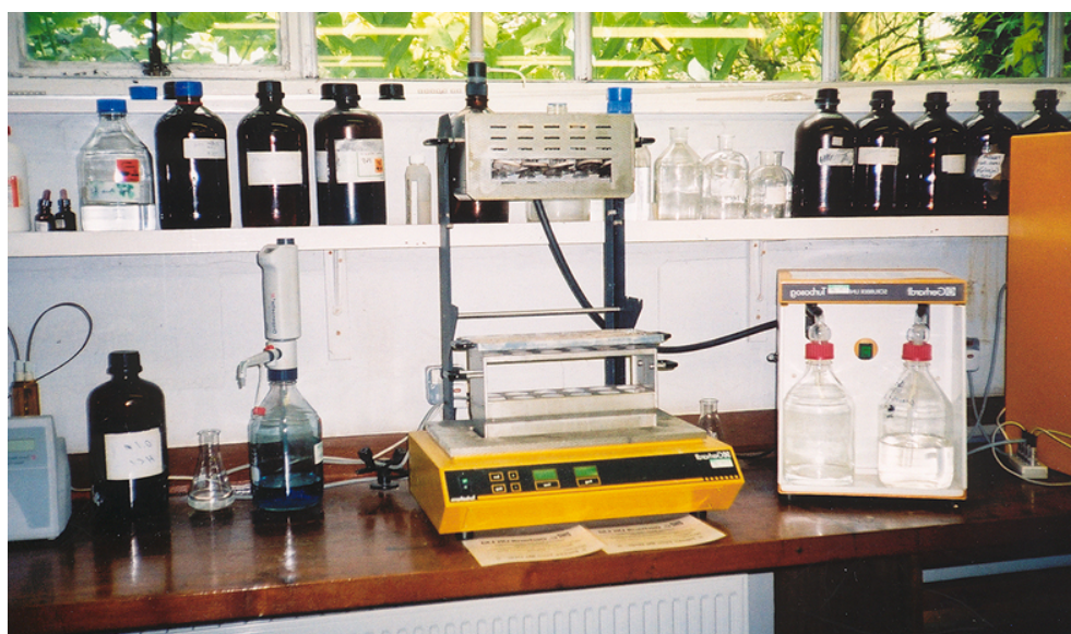
Plate 2.5. Kjeldahl digester along with the scrubber and titration unit.
