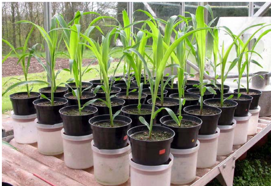
Plate 2.4. Pots arranged in individual plastic pots for leachate collection.
