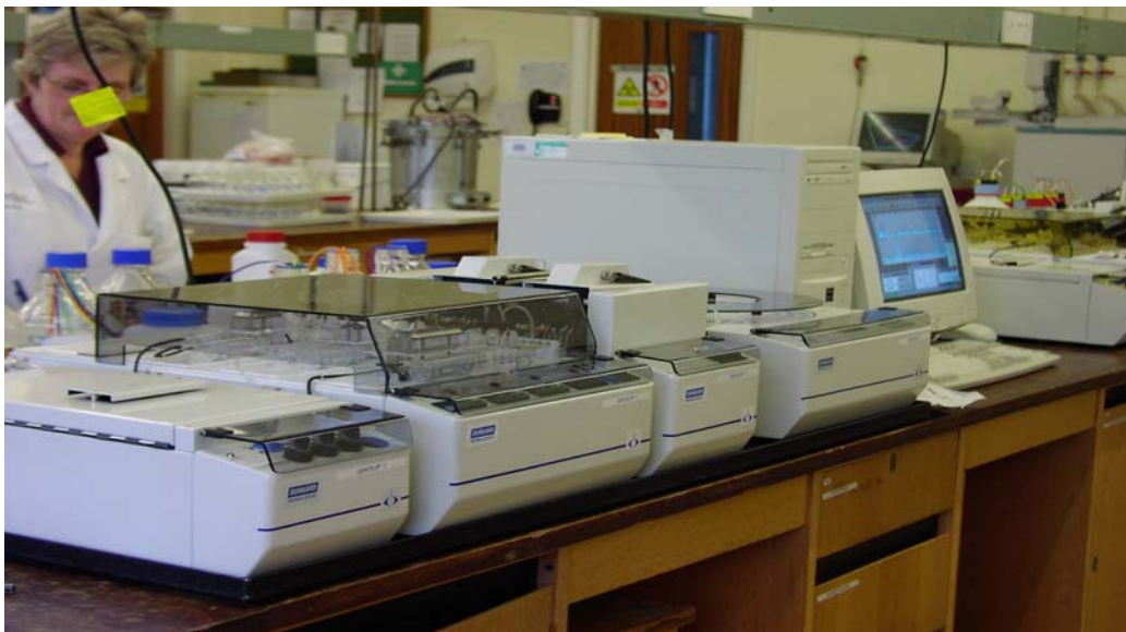
Plate 5.2 Segmented Flow Auto-Analyser.
