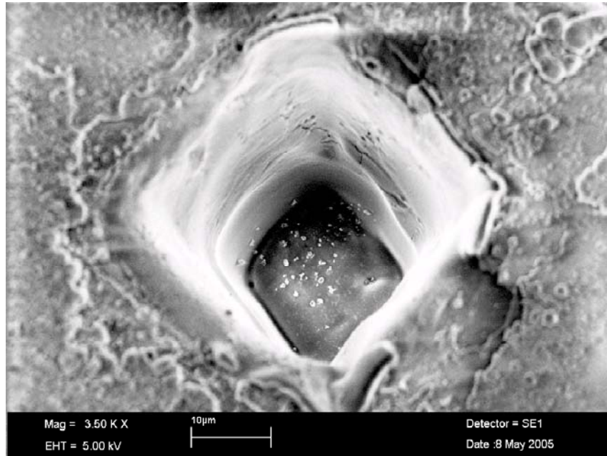
Figure 8-27: Sapphire ablated 24.5 \times 10^4 \text{ Jm}^{-2} at 5 Hz for 500 pulses.
