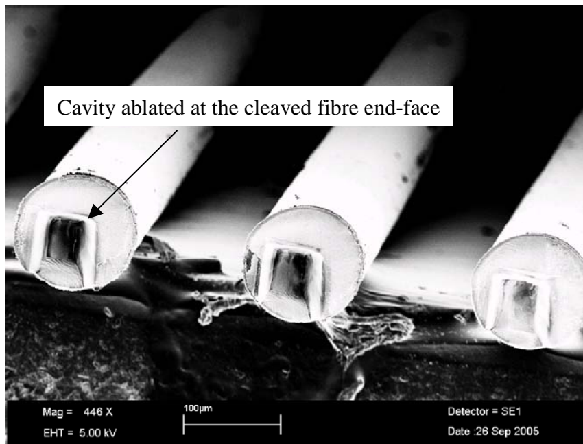
Figure 9-25: Ablated cleaved ends of the SM 800 fibre ribbon cable.
