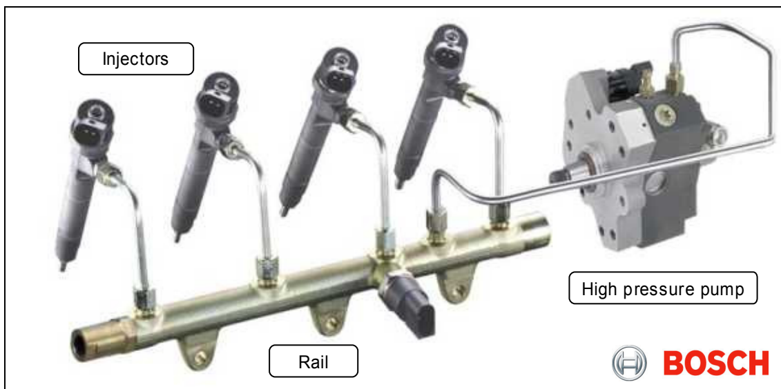
Figure 6.1: Common Rail System – Overview (BOSCH 2005g)
