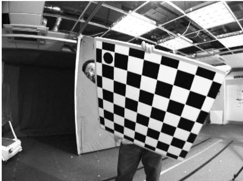
FIGURE 2.15: Tsai grid calibration pattern.
