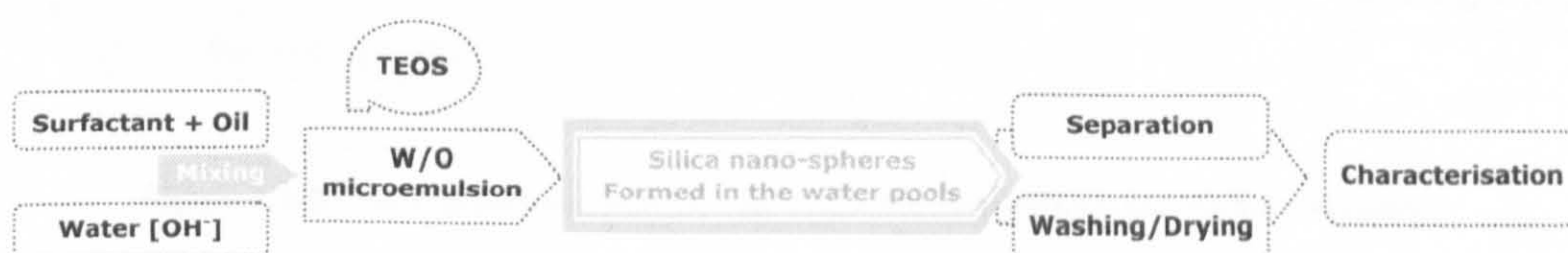
Figure 3.3-3 Flow chart of the synthesis of silica nano-spheres via w/o microemulsion system.
