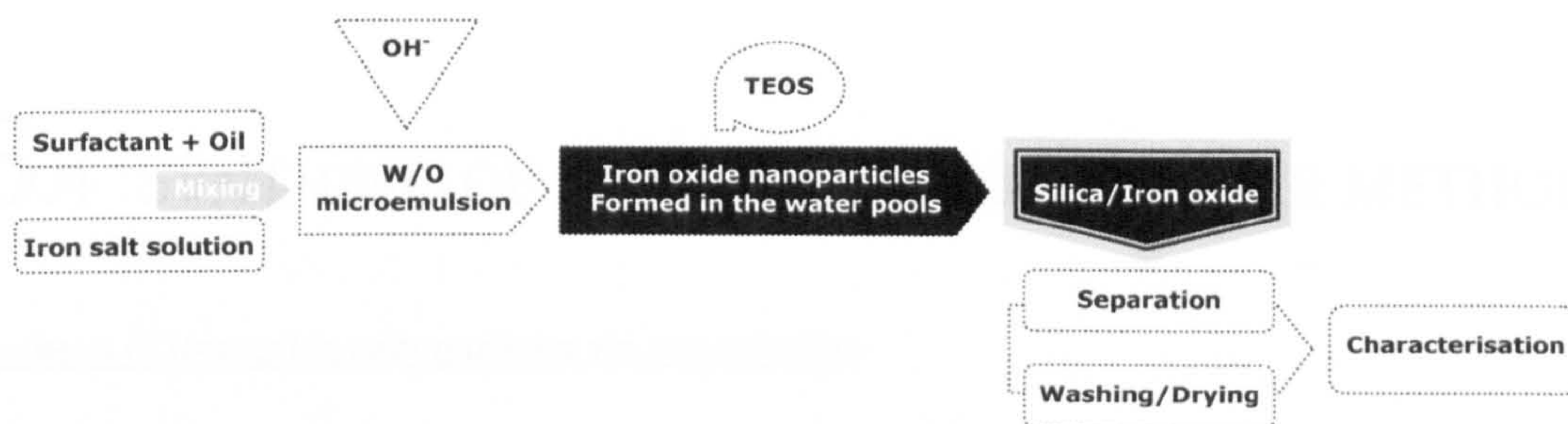
Figure 3.3-4 Flow chart of the synthesis of silica/iron oxide nano-composites via w/o microemulsion system.
