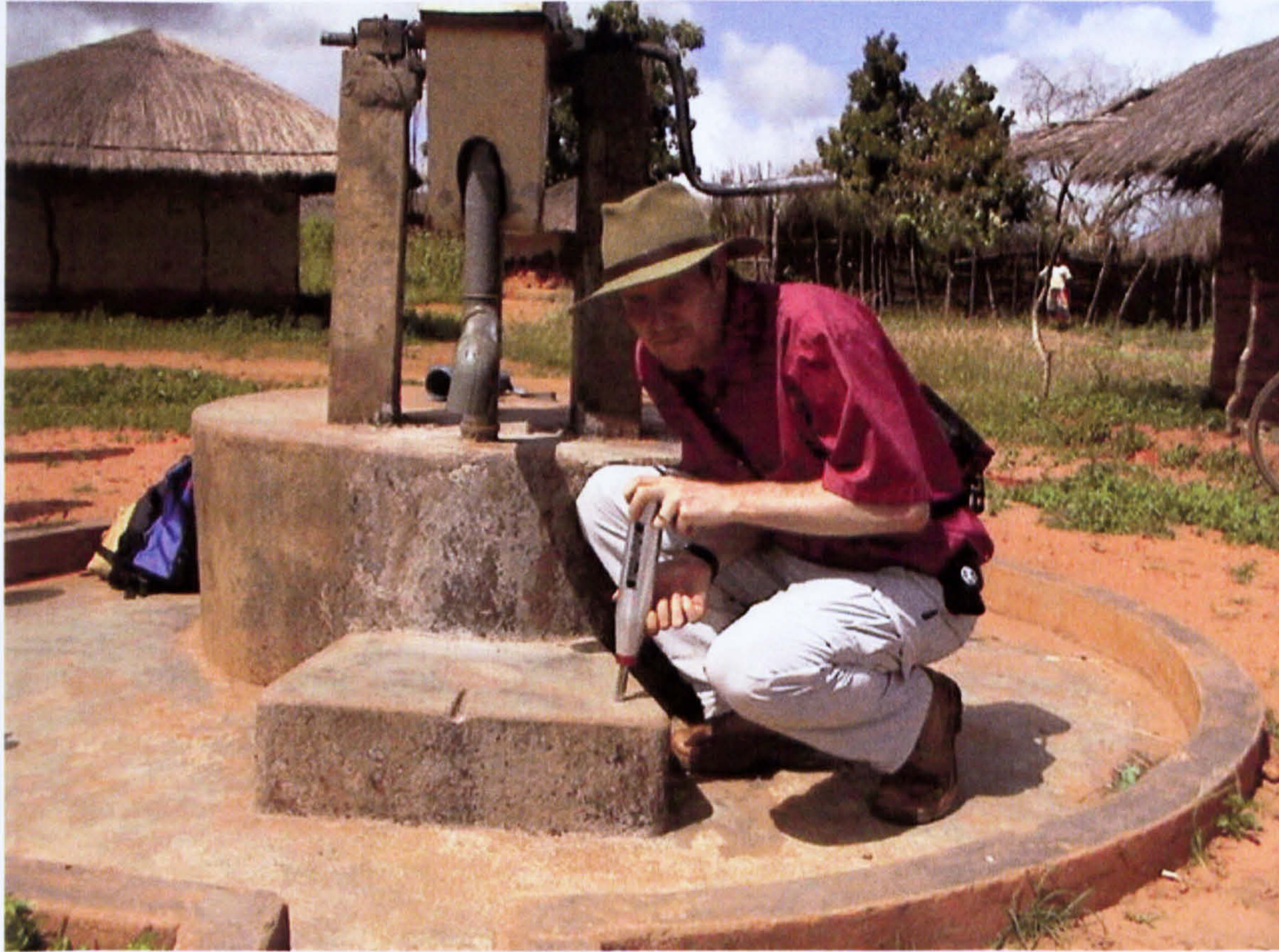
Figure 17: Surface Hardness testing by the author
