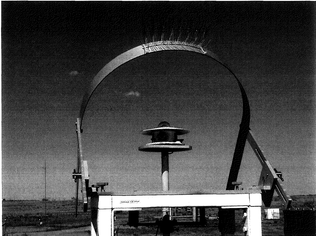
Figure 2.1 a. A battery of various Kipp & Zonen pyranometers. b. Kipp & Zonen pyranometer with shade-ring attached. (Courtesy of NREL, www.nrel.gov )
