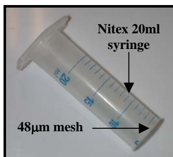
Fig. 3.2.7 An example of a 20ml Nitex mesh strainer used to separate sperm and eggs after specified contact times.
