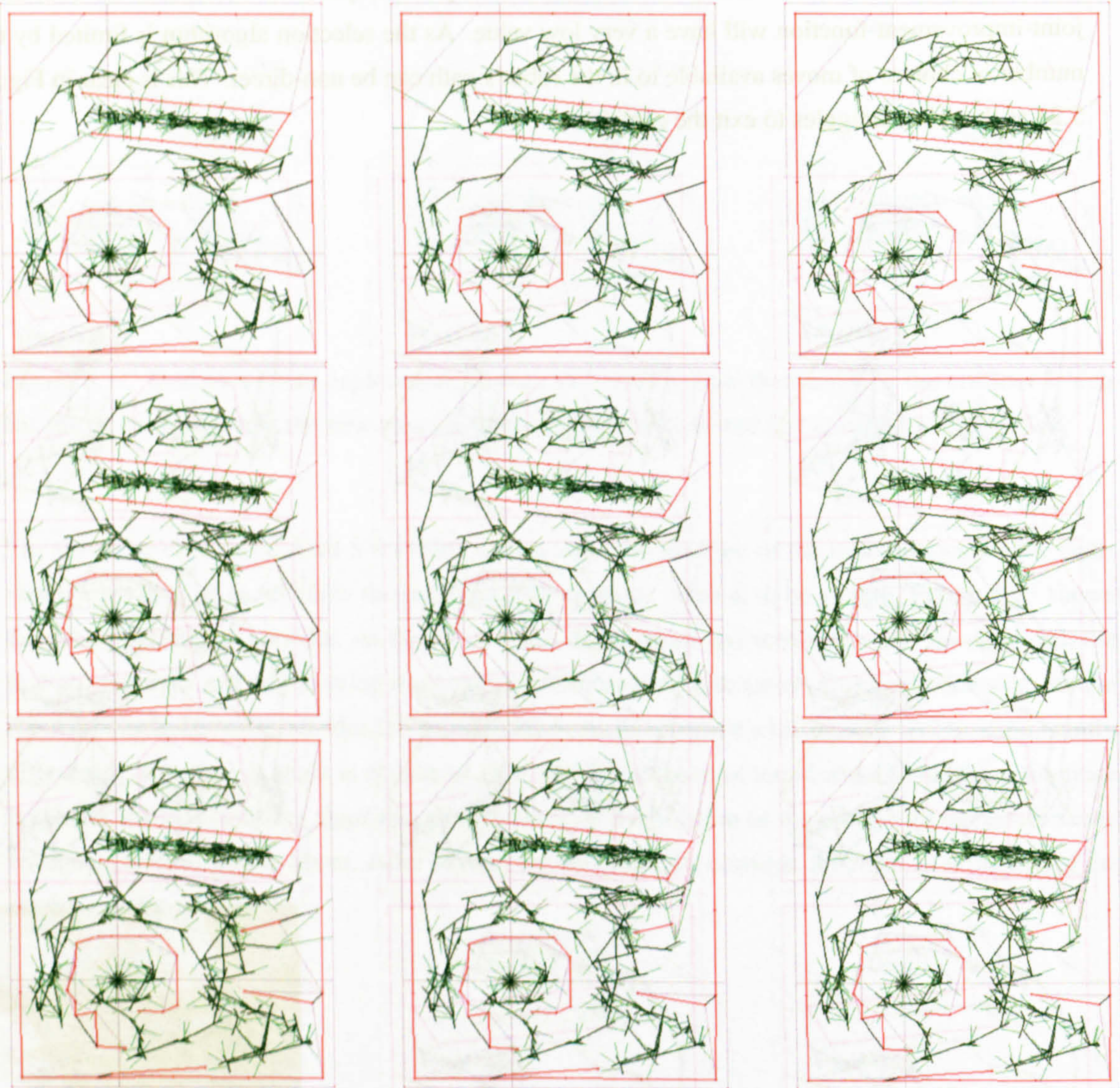
Figure 5.24: Complex room exploration: moves 290-2 as the robot exits the corridor, 316-7 as the robot moves back across the scene and detects a new area & 320-3 as the robot views the new area.
