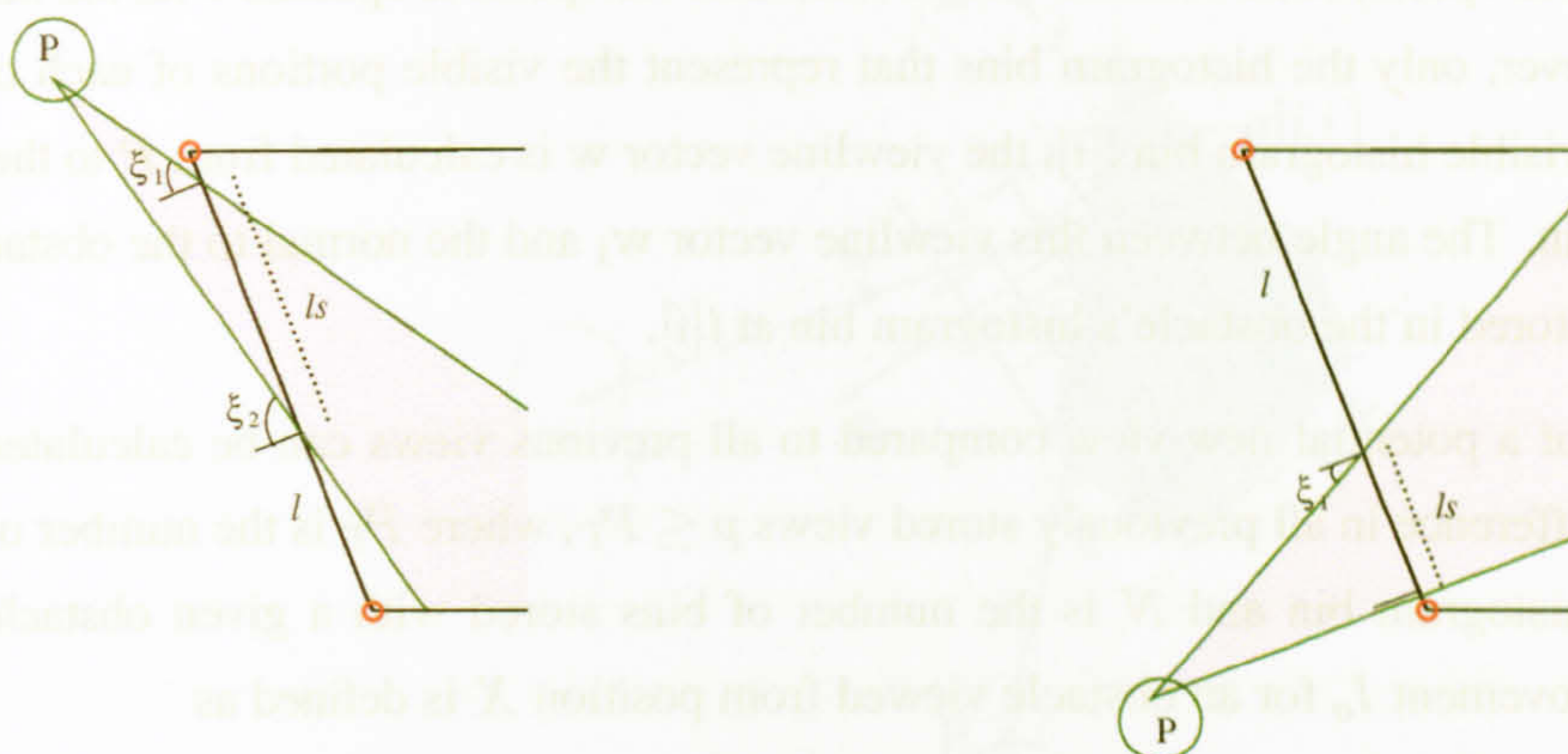
(a) The portion l_s of the obstacle l is visible from P , with viewed-from angles ranging from \xi_1 to \xi_2 .
