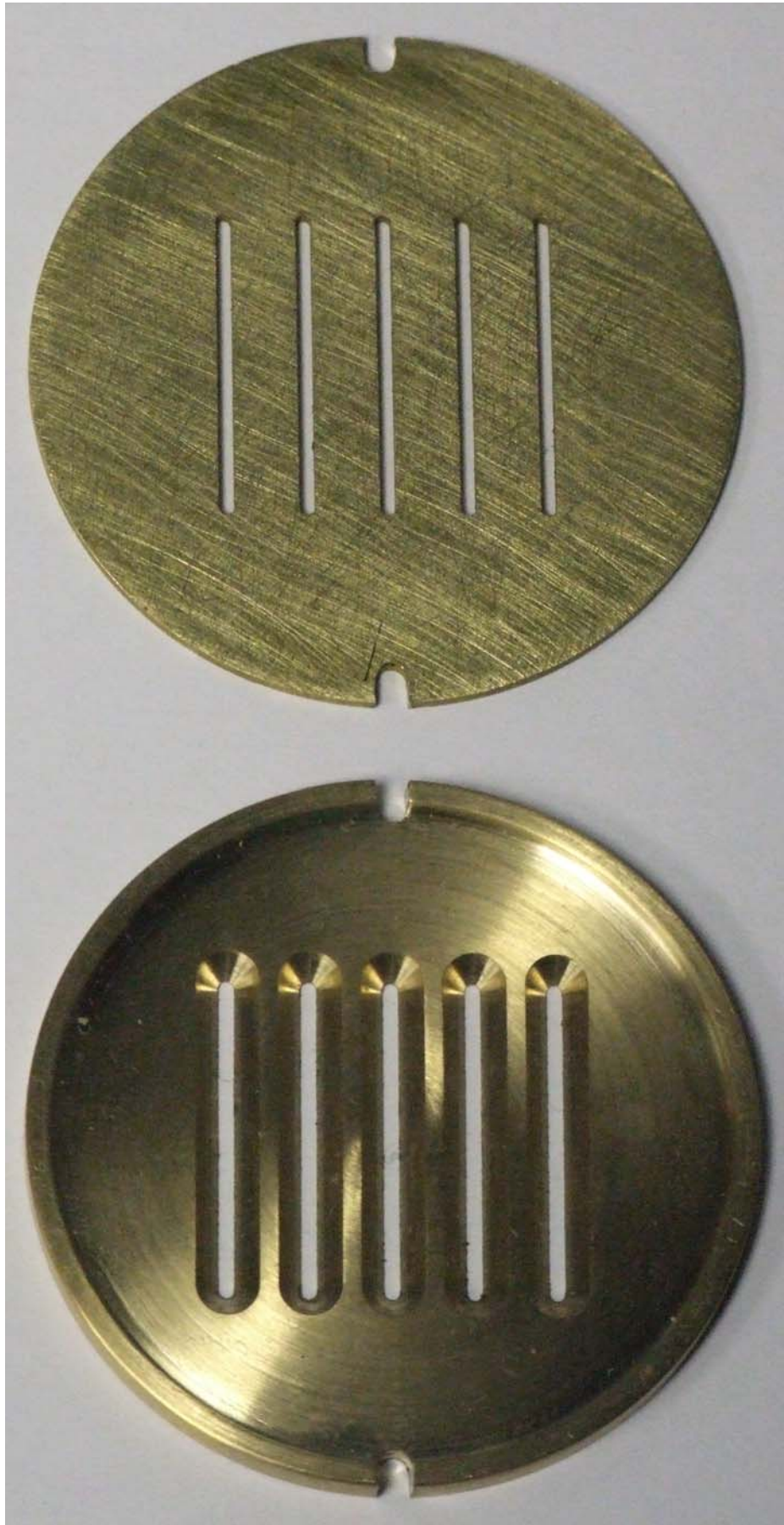
Figure I.3 Sample securing discs, sample holder disc (top) and sample clamp disc (bottom)
