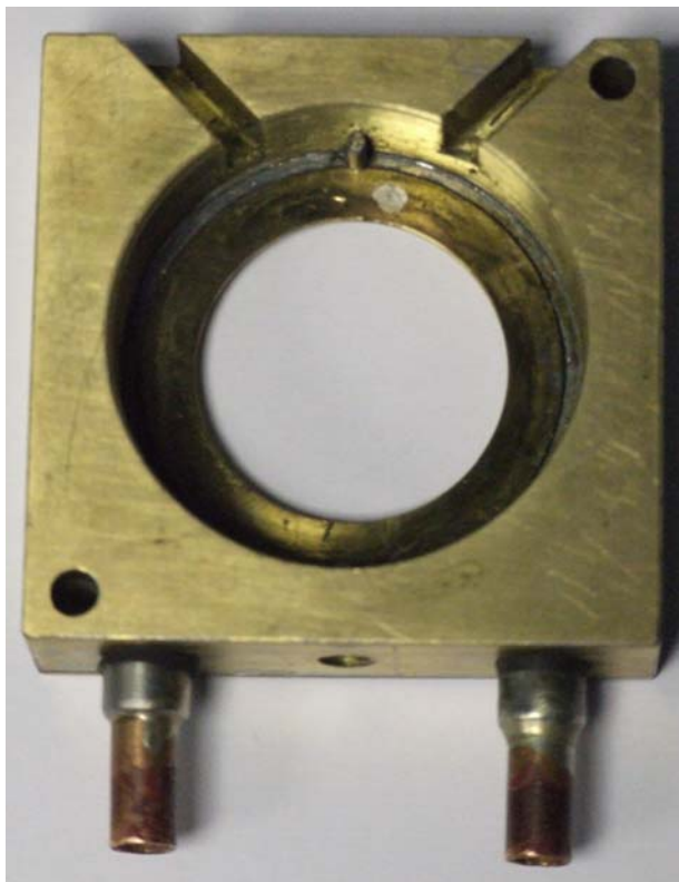
Figure I.2 Sample holder base unit designed by Dr S. Wilkinson
