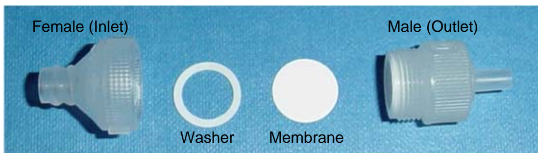
Figure 4.1 Swinnex Syringe Filter; Consisting of an inlet and outlet which are screwed together securing a membrane disc.
