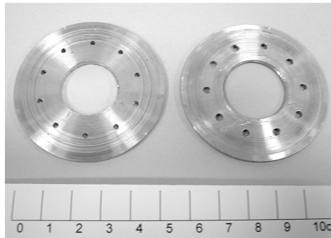
Figure 27 The baffles showing 2mm (left) and 3mm (right) holes
