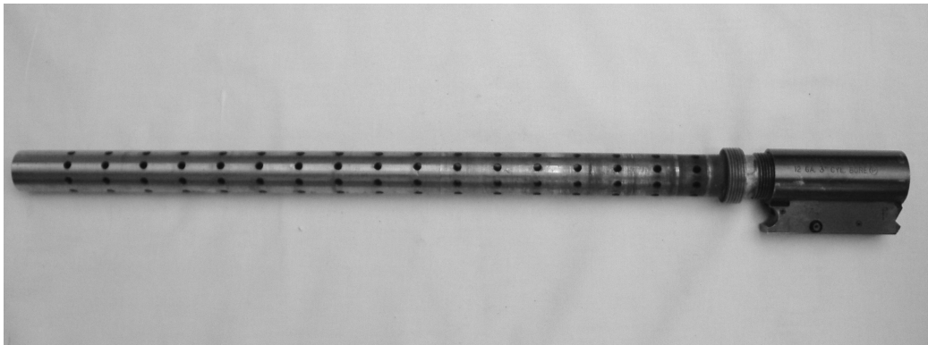
Figure 25 Experimental barrel showing the 4mm holes
