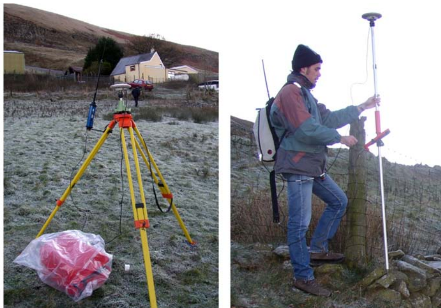
Figure 4.2. Leica System 500 receivers: base station on tripod (left) and rover antenna mounted on pole (right).
