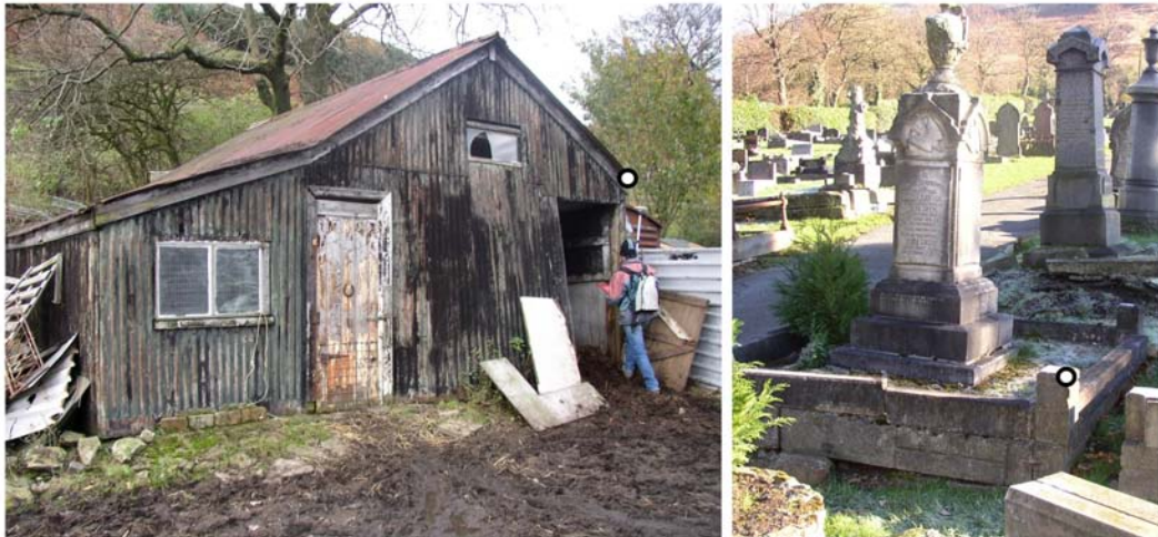
Figure 6.7. Typical targets for ground control: corner of an old barn and a gravestone.
