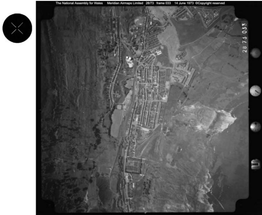
Figure 6.11. Frame 7333 of the 1973 epoch (© copyright reserved); the enlargement shows one of the uncalibrated fiducials.
