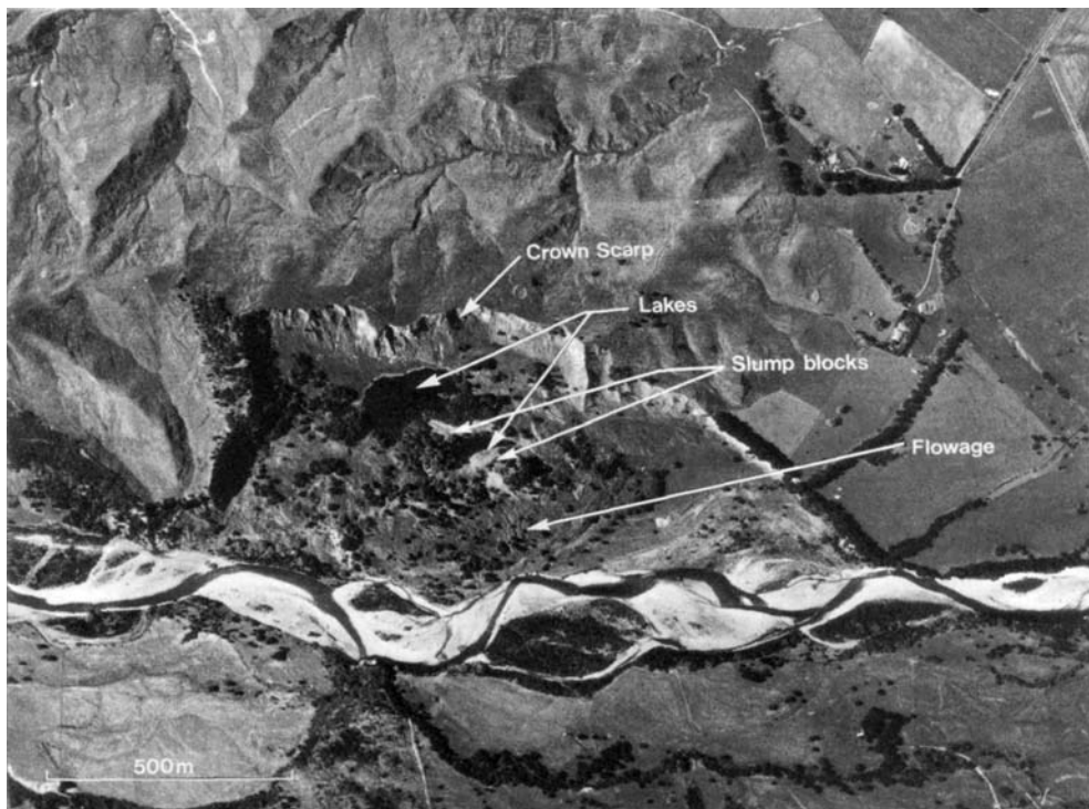
Figure 2.8. Aerial photograph of the Ruamahanga slump (New Zealand) showing some distinctive features (Crozier 1984).
