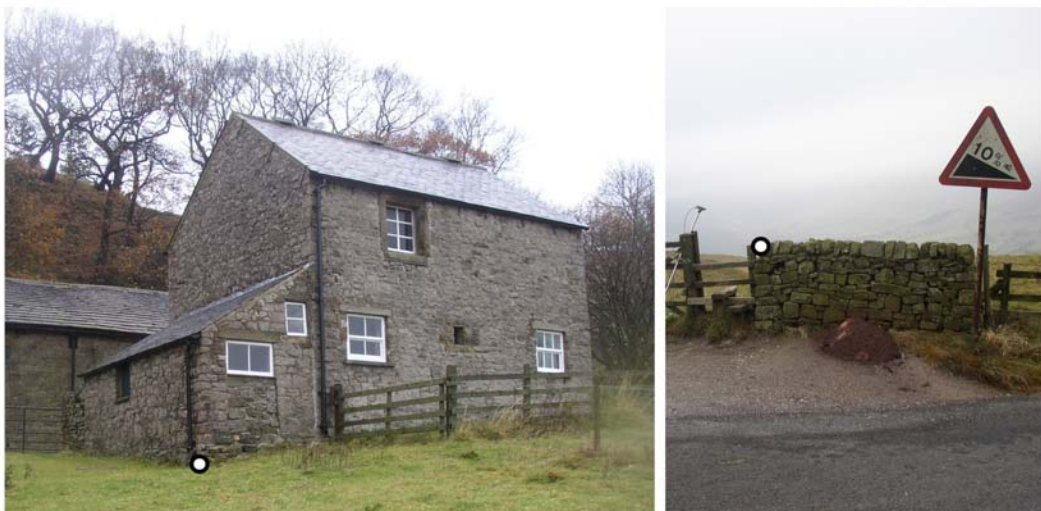
Figure 5.7. Typical targets for ground control: corner of a building and stonewall.
