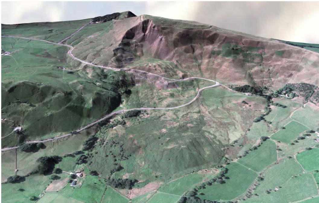
Figure 5.46. Realistic 3D view of Mam Tor, created by draping an orthophoto over a DEM, both acquired from the 1999 images.
