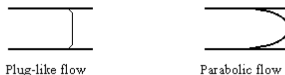
Fig. 16. Difference of the flow profiles in CE (plug-like) and HPLC (parabolic) with the force being applied all along the capillary and from one end of the capillary respectively.
