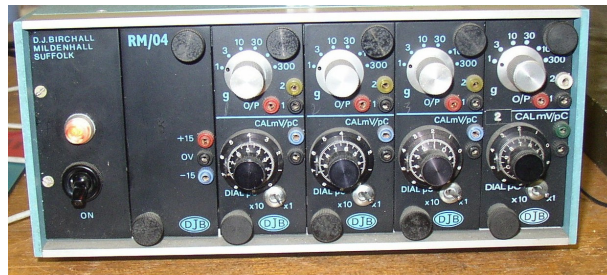
Figure 6-3. A charge amplifier
