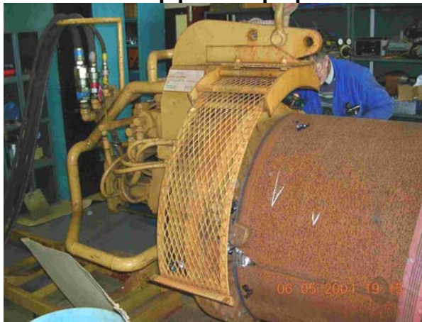
b) 36 in CRC pipe bevel preparation machine
