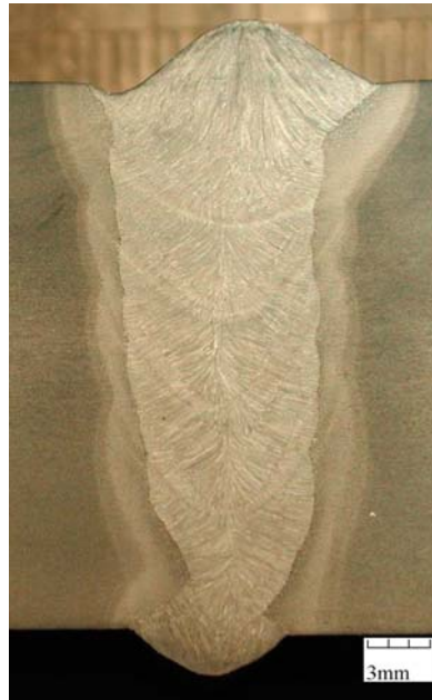
Fig. 6-20 Typical dual tandem double joint procedure (DJ-DT-N012) macro section
