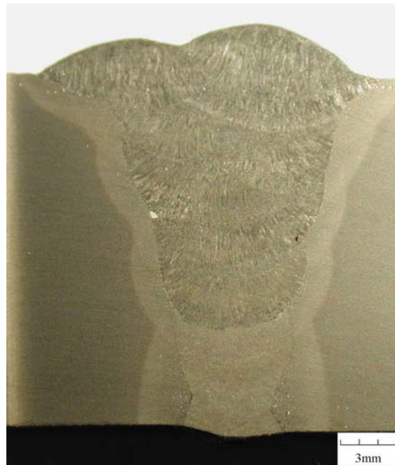
Fig. 6-27 Typical Tie-In procedure (Tie-In S01) macro section
