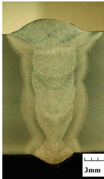
Fig. 6-6 Typical dual tandem procedure (ML-DT-S016) macro section
