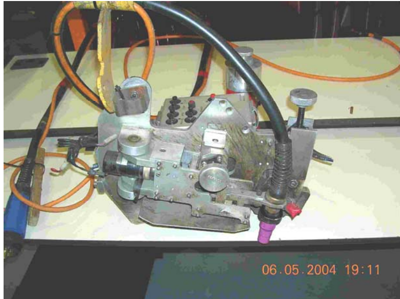
Fig. 4-12 CRC-Evans P100 welding carriage and single wire air cooled torch
