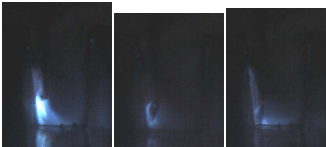
Fig. 7-20 Arc and droplet transfer at the minimum (0.3mm) wire distance from the sidewall (run No. 4 of the experimental design)
