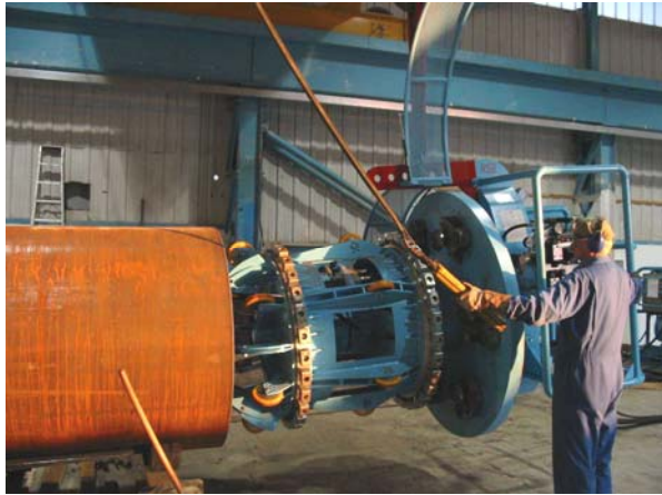
a) 52 in BROOKS pipe bevel preparation machine
