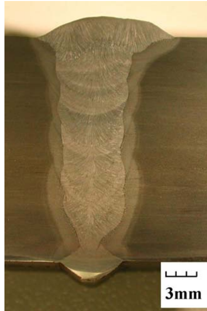
Fig. 6-9 Typical dual tandem low carbon procedure (ML-DT-N009) macro section
