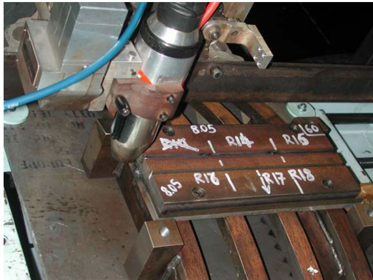
Fig. 5-9 Plate bevel preparation and experimental setup
