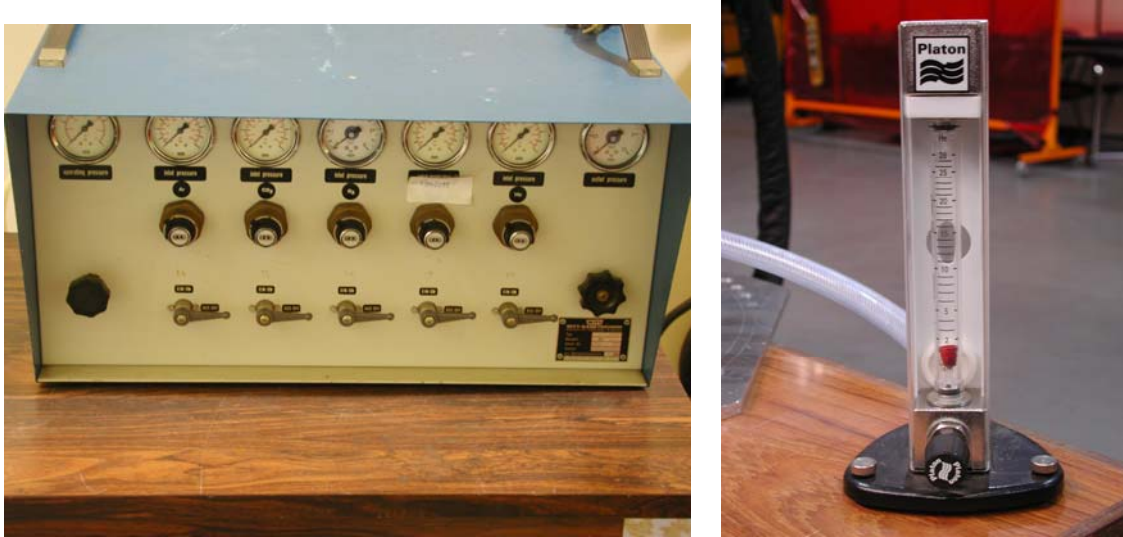
Fig. 4-1 The Witt KM-S gas mixer and Platon Gasmeter type GTLK gas flow meter
