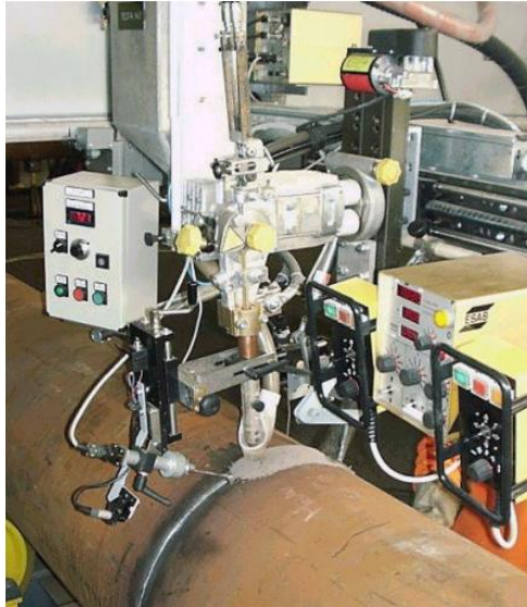
Fig. 2-6 Twin arc heads for pipeline SAW welding (photo courtesy ESAB UK)
