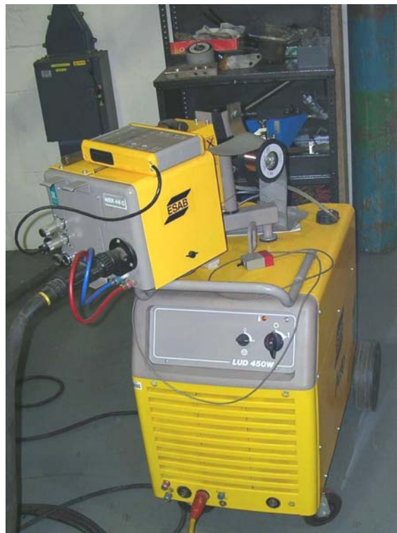
Fig. 4-8 The ESAB Aristo LUD 450W and the associated wire feeder
