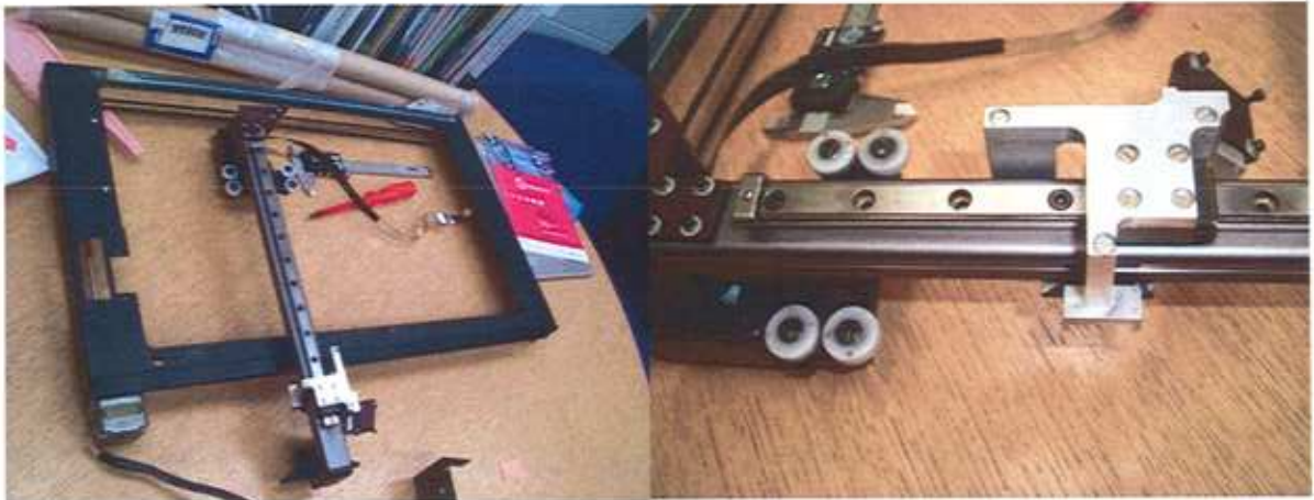
Figure 6.4.9.1 - LOM Laser guide (plotter), Y axis linear bearing and X axis old roller bearing
