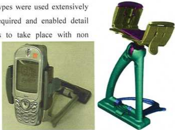
Figure 6.4.7 - SLA RP of Holder with phone and CAD design rendered
