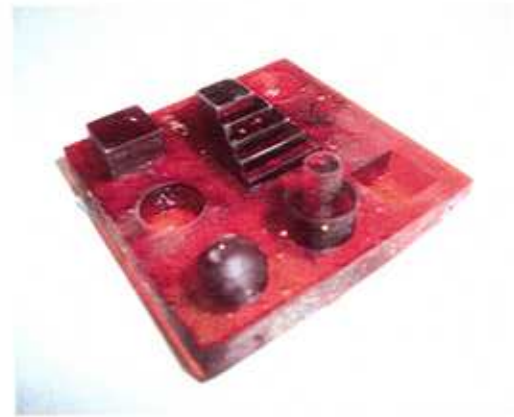
Figure 3.6.2.3 – CAD Geometry test piece and sample produced
