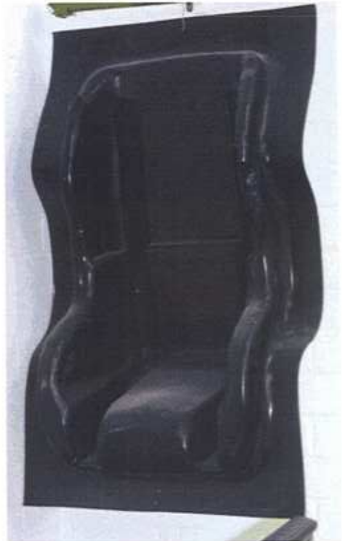
Figure 6.5 - Thermoformed child car safety seat from LOM mould tool
