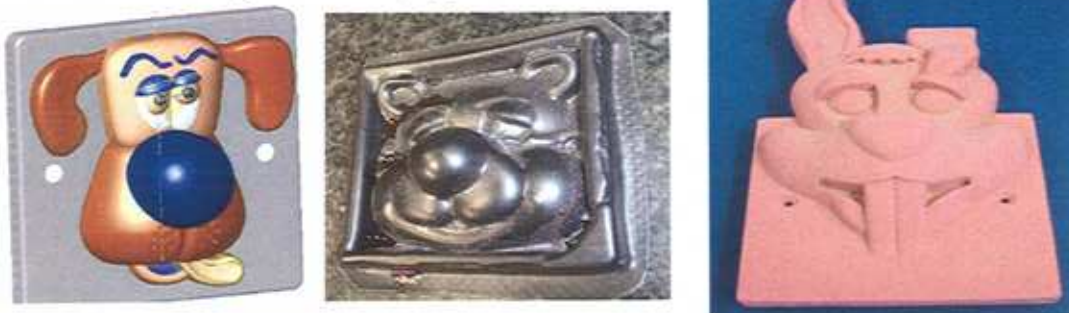
Figure 6.4.6 Teddy bear light switch Vacuum formed and Rabbit 3DP part
