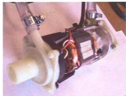
Figure 6.3.1 - SLS manufactured LP Hydroplane on test and SLA built new pump configuration
