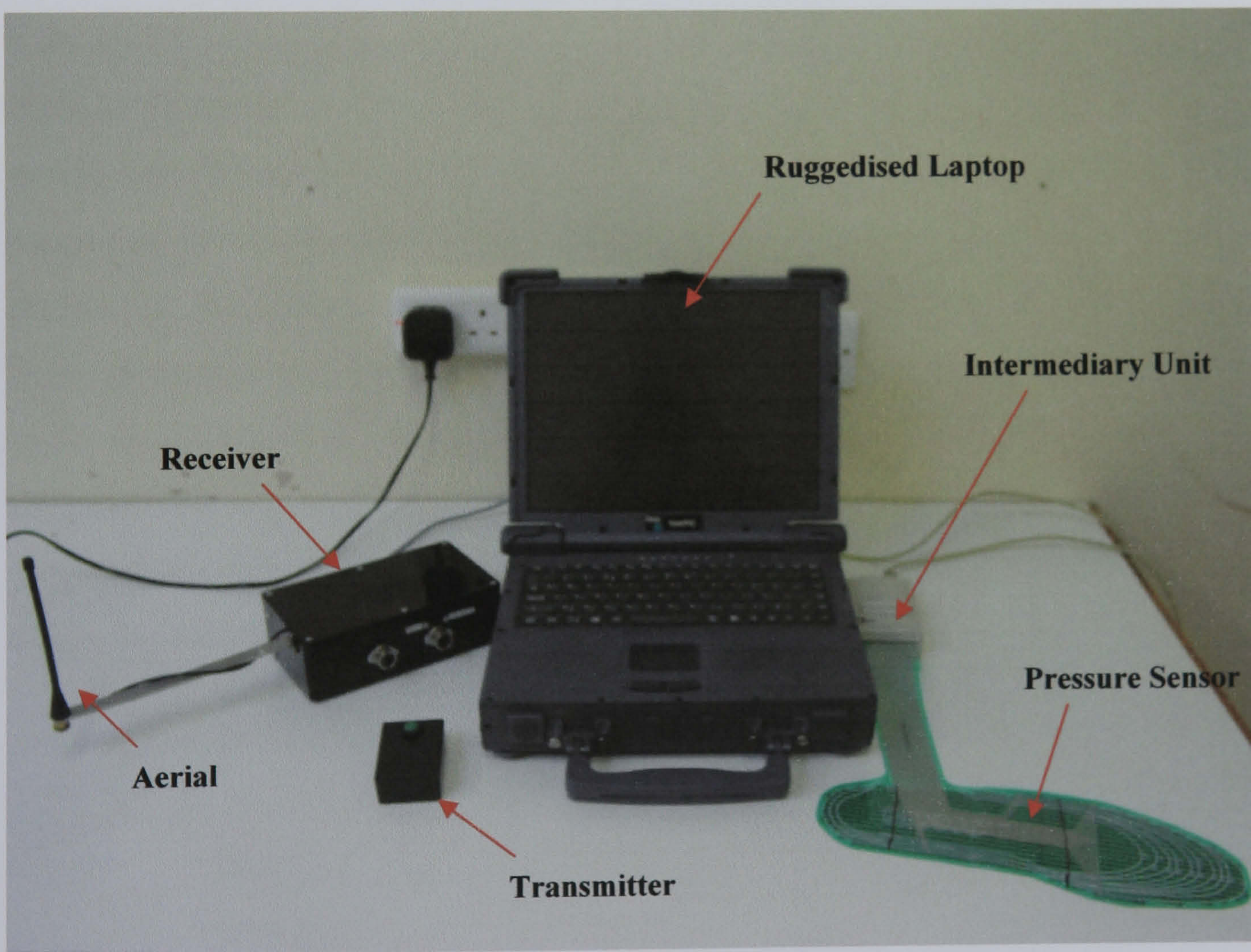
Figure 4.4 The remote trigger and associated field equipment
