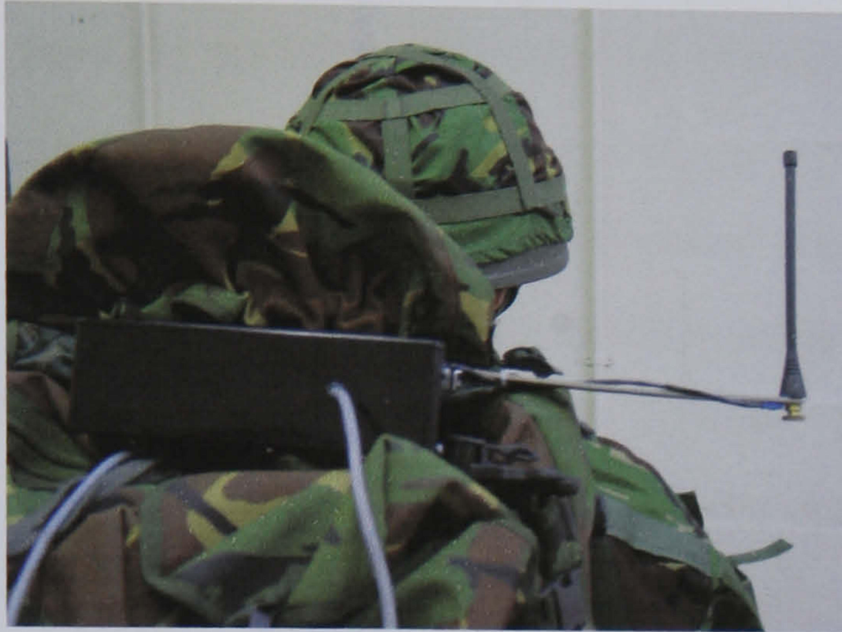
Figure 4.5 and 4.6 The trigger receiver connected to the computer (inside the backpack). The aerial can be seen prior to placement in the backpack (4.5) and in situ (4.6).
