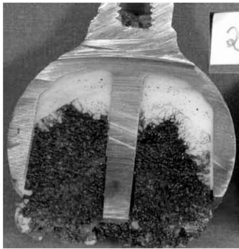
Fig. 5 Low-viscosity cement: incomplete seating
