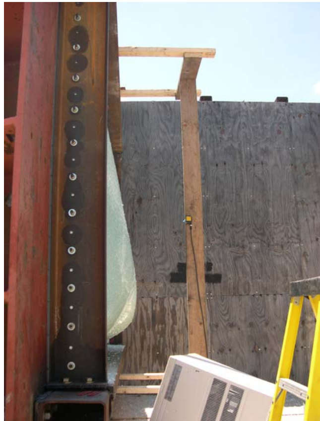
Figure 226. Laser sensor and test cubicle, with panel 3 after test
