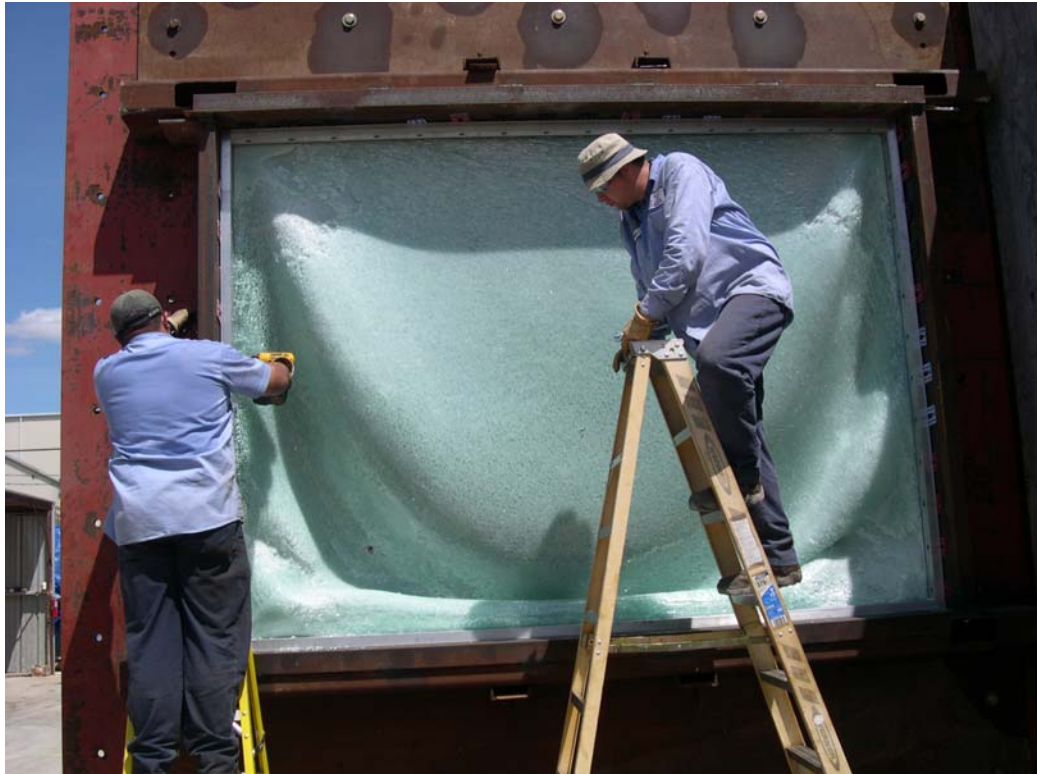
Figure 223. Typical cracked Panel 3 after test in the shock tube
