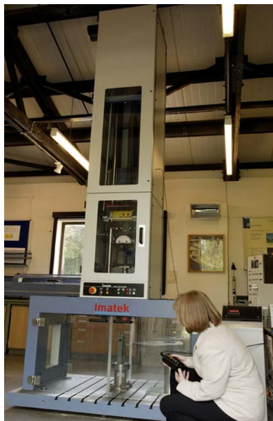
Figure 124. The Imatek impact testing machine at Cranfield University DCMT Shrivenham
