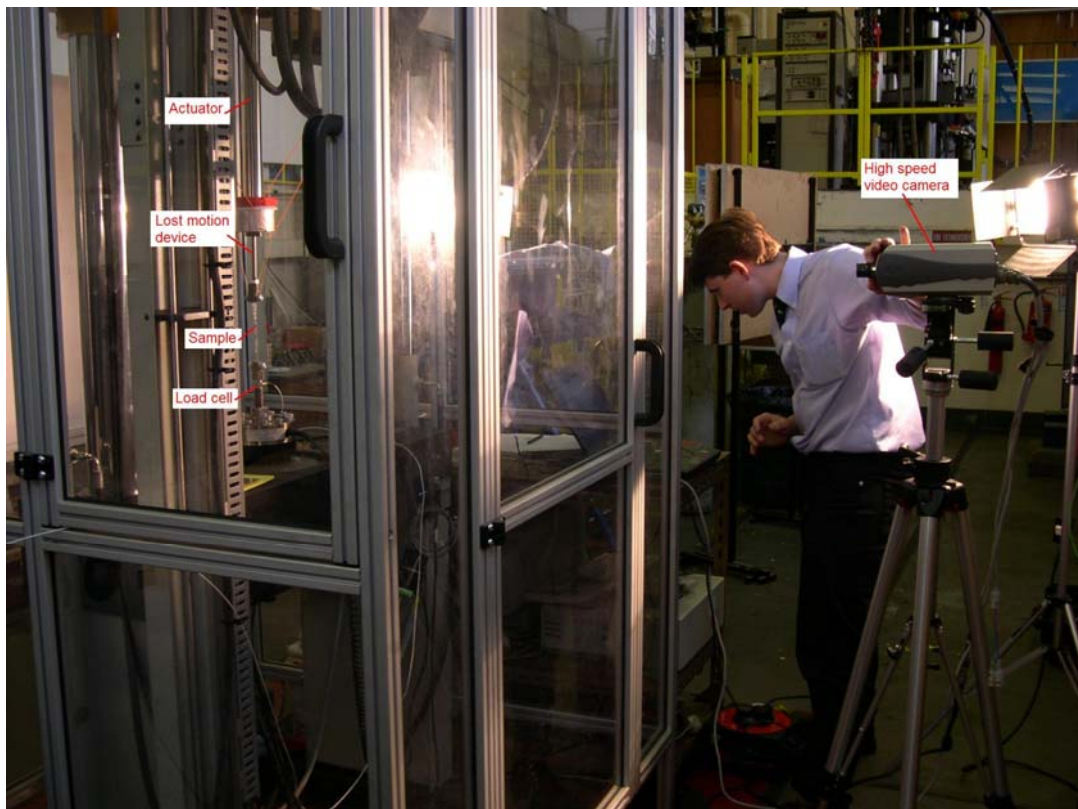
Figure 143. Instron test actuator and safety cubicle, with video equipment
