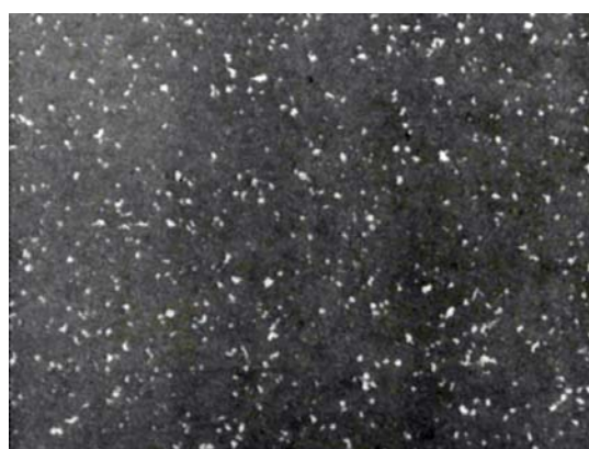
Figure 4.2 Alumina microstructure image after inverting pixel grey level
