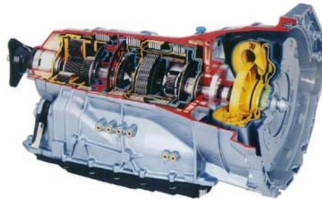
Figure B.161 – ZF 6HP26 6-speed automatic transmission [B.4]. In production since 2001, the torque capacity is in excess of 600 Nm within an overall ratio spread of 6.05.
