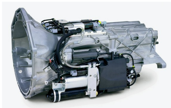
Figure B.167 – Automated sequential gearbox SMG [B.10]. With 11 control modes and a launch control function, this AMT shifts as quickly as 80 ms in its most aggressive mode.
