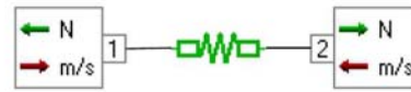
Figure C.174 – Simple 1D model of a spring [C.1] where all side loads are ignored
