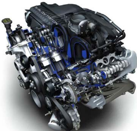
Figure 4.45 – Ford Triton 5.4 V8 gasoline engine cut-away. Shown here in its 3 valve per cylinder configuration the engine is a naturally aspirated.
