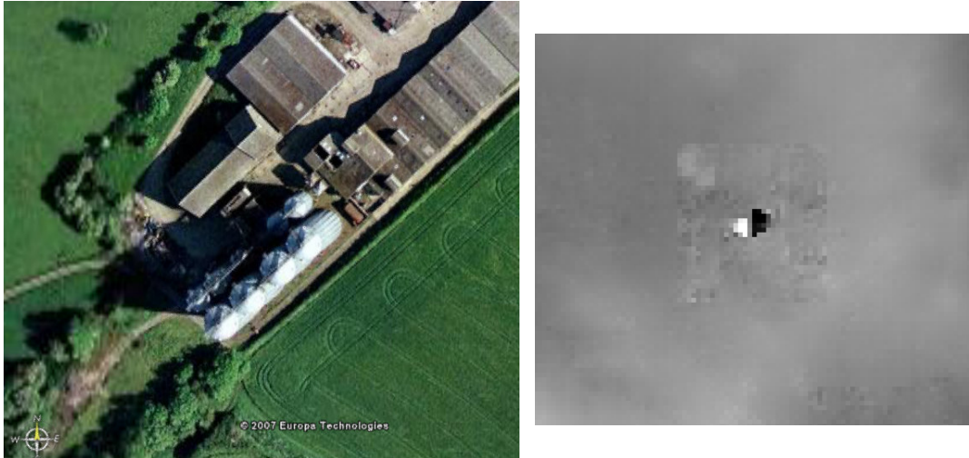
Figure 4-16. Left: aerial view of disused grain silos located on Station road, Turvey, Bedfordshire (UK) (Google Earth, 2007; with the education setting reproduction agreements). These buildings are 30 m high Bedford Borough Council (2007). Right: height computed with the first ERS interferometric tandem pair (i.e. 25 th and 26 th June 1995). The phase unwrapping algorithm is not able to successfully compute an accurate height of these structures. The two images have a different scale and orientation, and are presented for illustration purposes only.
