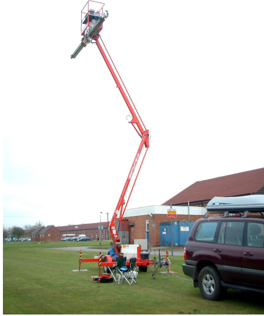
Figure 4-26. GB-SAR system deployed at a height of 10 m. The antenna incidence angle \theta is set a 45^\circ . The weather station has not been installed.
