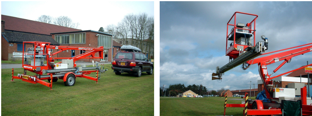
Figure 4-25. Left: GB-SAR stowed configuration. The 4-wheel-drive vehicle is used to transport it and house the majority of the instrumentation. Right: GB-SAR set-up, with the hydraulic lift not deployed and the C-band antennas pointing horizontally
