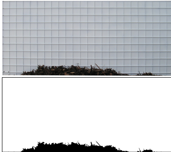
Figure 4-3. Modification of the brightness and contrast of the profile images to obtain a black and white image only.
