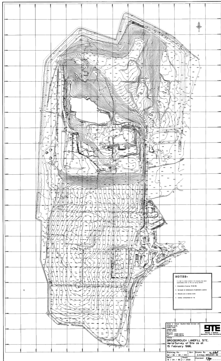
Figure 5-23. Topographic survey with a 100 m spacing grid of Brogborough landfill provided by Waste Recycling Group Ltd. 15 th February 1996. These surveys specify the exact location of the tipping areas and the presence of any lagoon used to monitor run of water or the presence of leachate.
