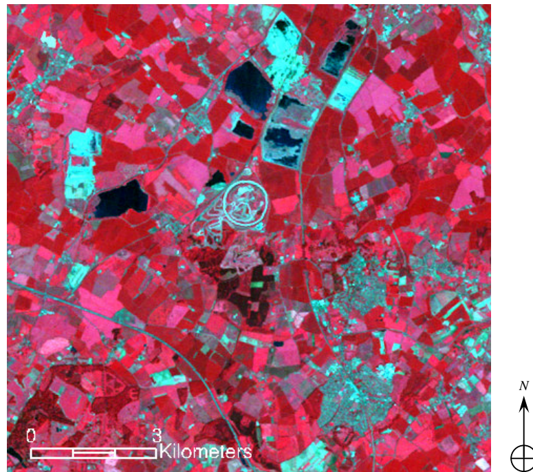
Figure 5-6. Landsat 5 TM sub-scene of Bedfordshire with 30 m ground resolution acquired 12 th June 1992. The image is obtained with a standard false colour composite with Band 2 (wavelength from 0.525 to 0.605 \mu\text{m} – green) as Blue, Band 3 (0.630 - 0.690 \mu\text{m} – red) as Green, and Band 4 (0.75 - 0.90 \mu\text{m} – NIR) as Red. The image is centred at 52° 2' 12'' N and 0° 31' 53'' W as Figure 5-5. Its printed size appears smaller than Figure 5-5 due to the coarser spatial ground resolution. Copyright University of Manchester/University College London Year 2001 (Landmap, 2005). Original Landsat 5 distributed by Infoterra International.
