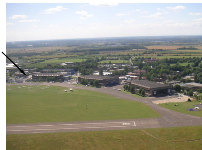
Figure 4-13. Aerial view of Cranfield University. The arrow identifies the selected feature with constant scattering characteristics used as centre when cropping the SLC.
