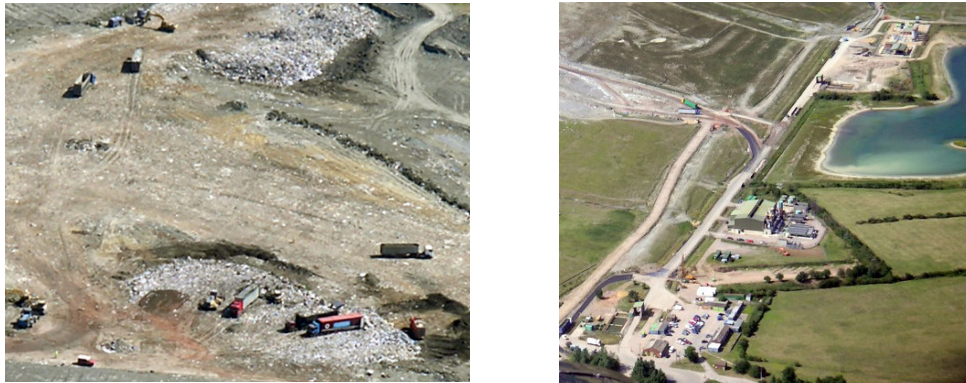
Figure 3-5. Brogborough landfill. Left: a variety of trucks continuously operate in the open cells (i.e. tipping areas) to deposit and compress the waste. Right: site buildings might include offices, power stations, storage buildings, and truck maintenance buildings (11 th July 2005).
