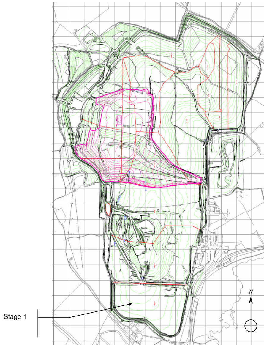
Figure 3-3. A survey map of the Brogborough landfill developed in November 2004. The grid is spaced at 100 m. The pink contour represents the operational void where open cells are located. Stage 1 is the selected area for ground observations of a fully restored cell. (Courtesy: Waste Recycling Group Ltd.)
