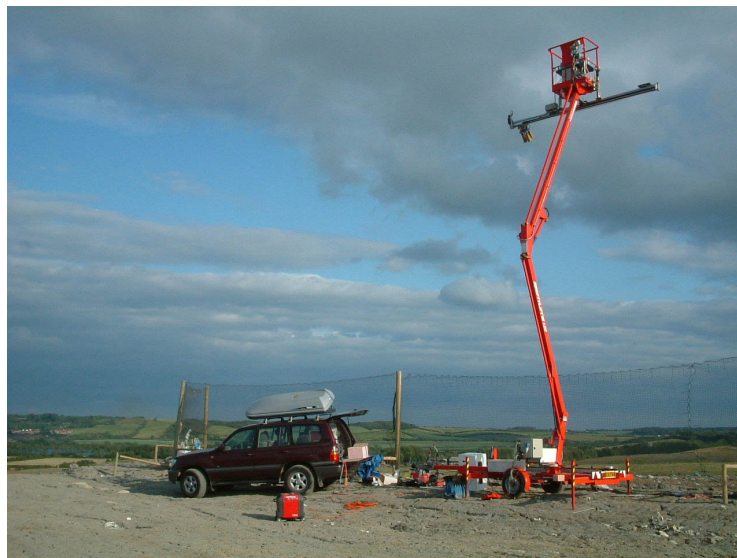
Figure 6-1. GB-SAR deployed configuration at the Brogborough landfill.
