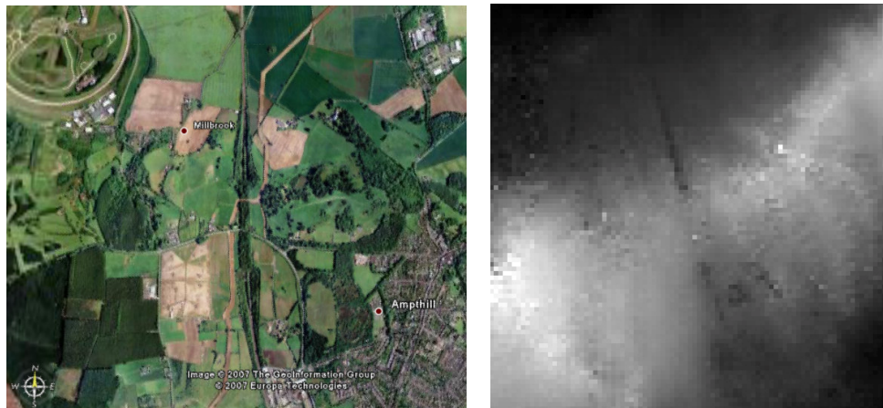
Figure 4-15. Left: aerial view of the Bedford-Luton (UK) train line tunnel between Milbrook and Amphill (Google Earth, 2007; with the education setting reproduction agreements). The height step change before the train enters the tunnel is roughly equal to 12 m. Right: height computed with the first ERS interferometric tandem pair (i.e. 25 th and 26 th June 1995). The average computed height at the two exits is 11.5 m. The two images have a different scale and orientation, and are presented for illustration purposes only.
