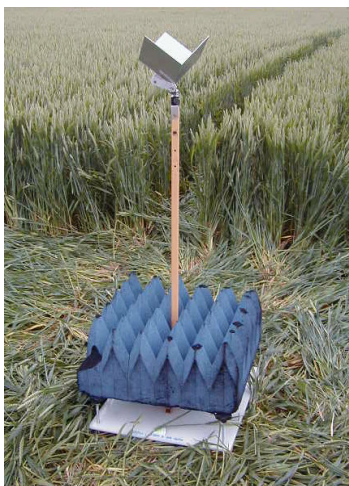
Figure 4-29. Levelled trihedral position at nadir at a height of 1.3m.
