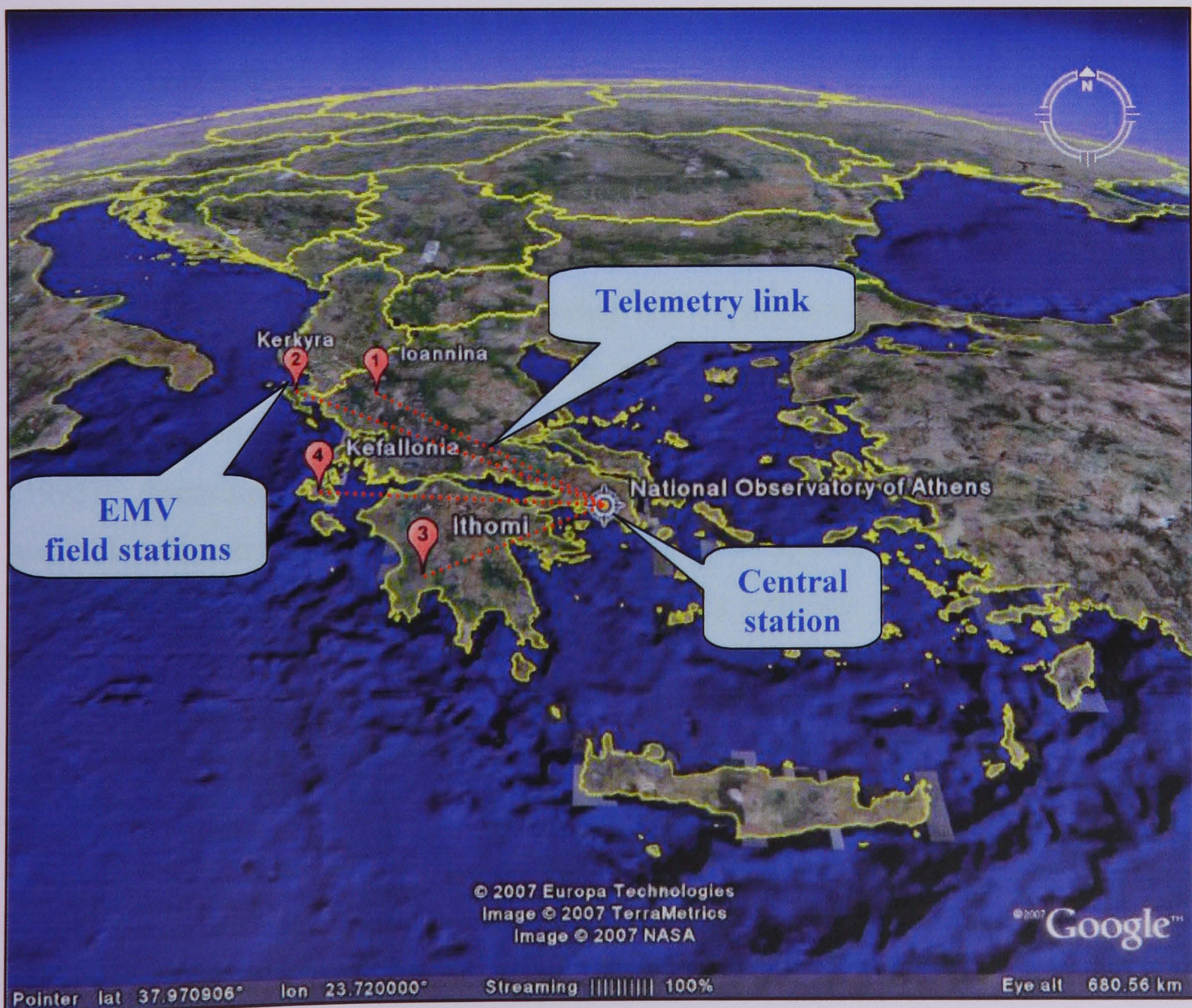
Figure 4.1 - Map of prototype EMV telemetric network in VHF band
