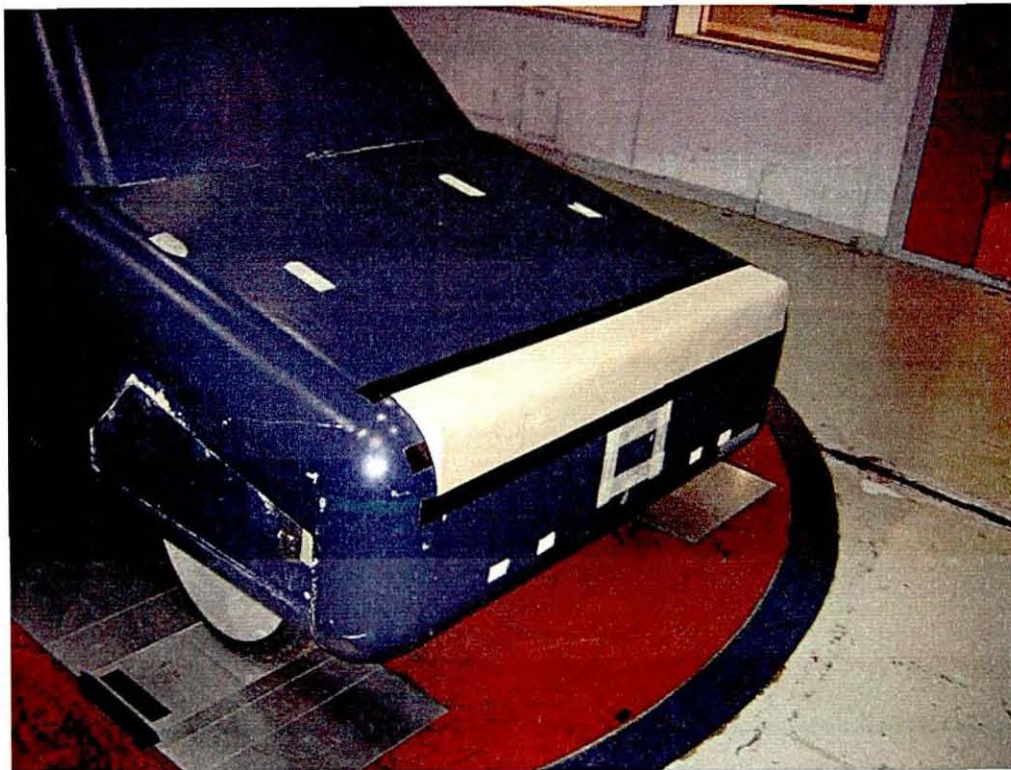
Figure 94 MIRA reference vehicle with leading edge radius modification fitted in the MIRA full scale tunnel
