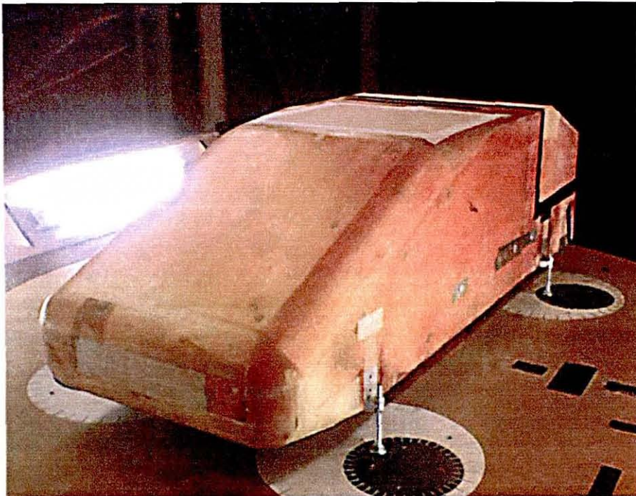
Figure 106 The Windsor model installed in the Loughborough model scale tunnel
