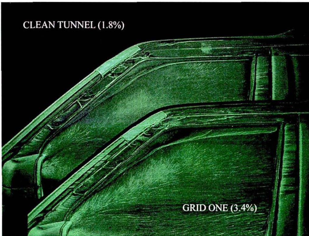
Figure 145 Fluorescence visualisation of A-pillar vortex, 1.8% turbulence vs. 3.4%
