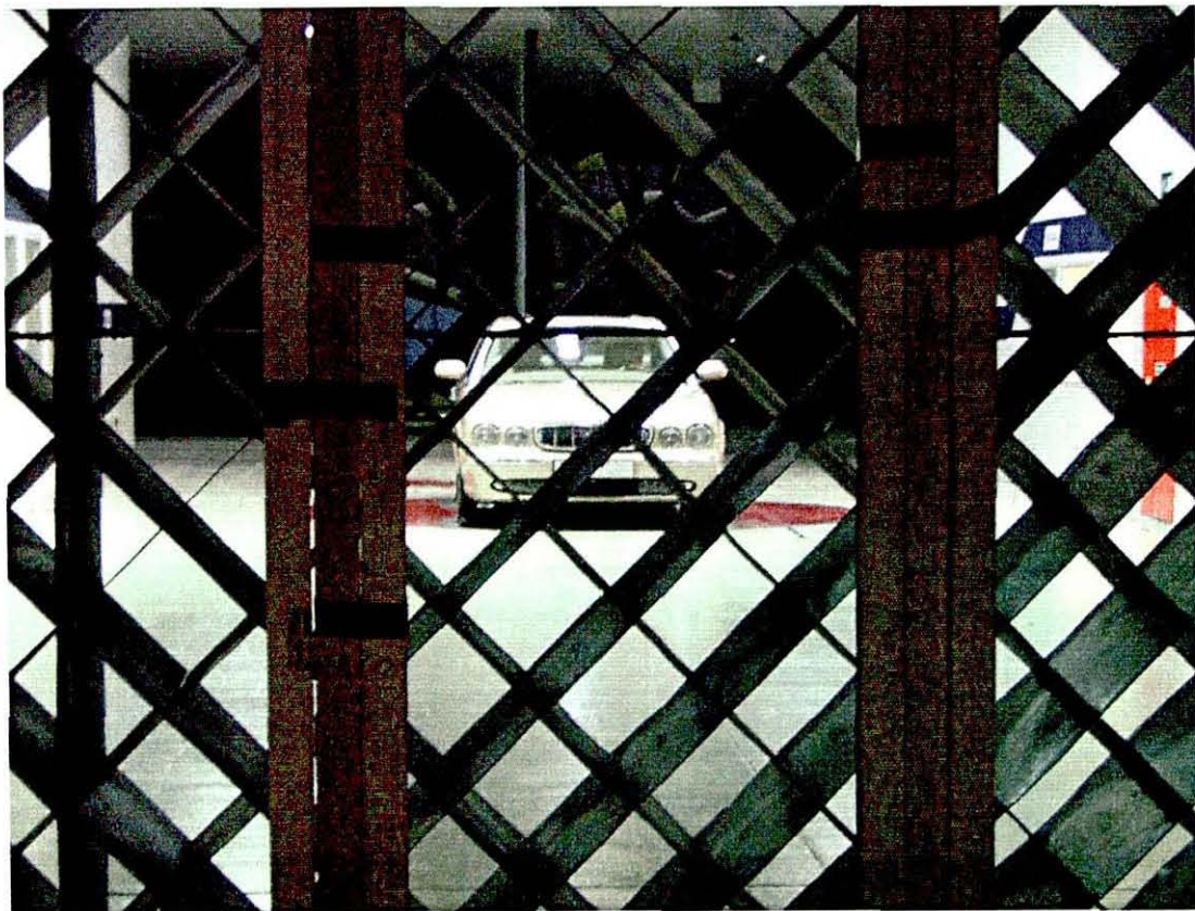
Figure 128 Jaguar XJ8 (X350) in the MIRA full scale wind tunnel, with the turbulence grid installed
