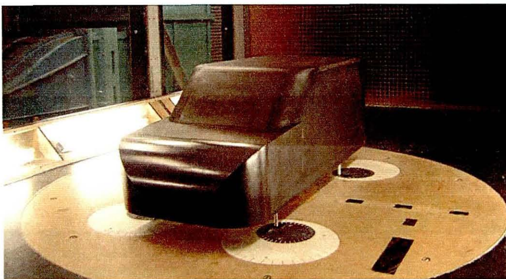
Figure 88 2-box model mounted in the Loughborough wind tunnel
