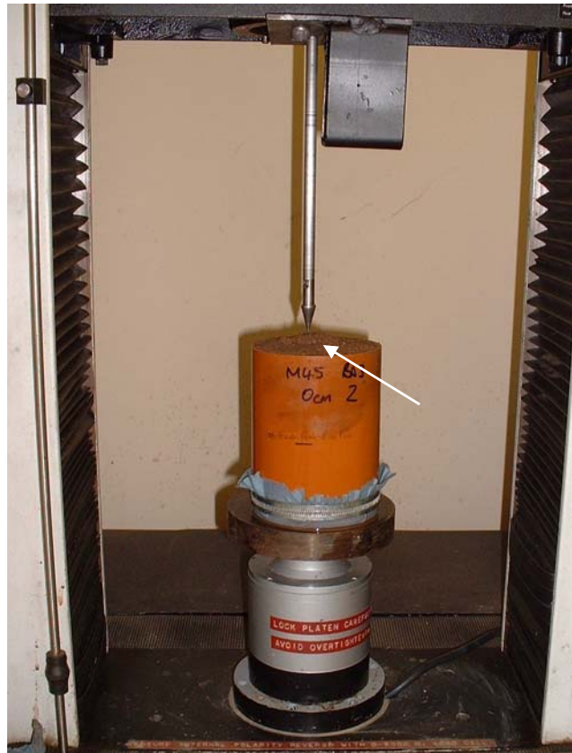
Figure 3.15 A NG cylinder on the Instron loading machine. (The arrow indicates a swell of particles on the soil surface as a result of upwards movement)
