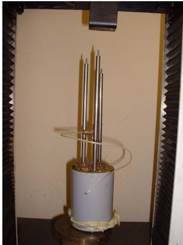
Figure 3.16 WG cylinder testing; three penetrometers and the tensiometer are visible.
