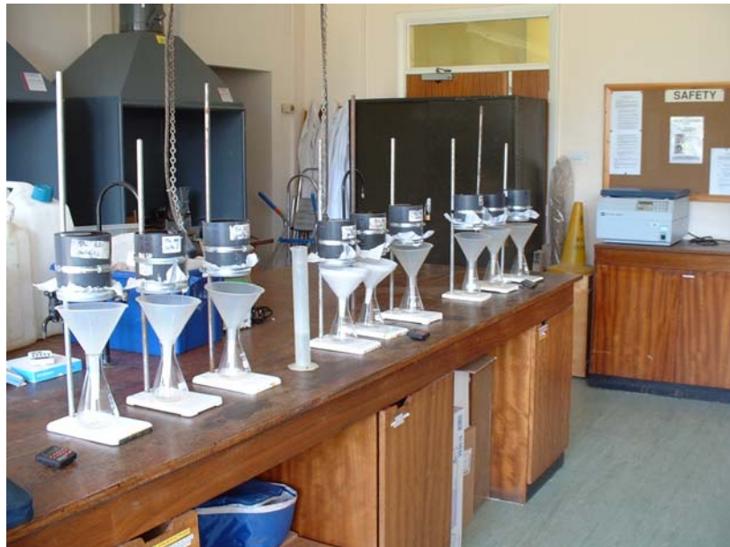
Figure 1 Cylinders of each soil type, supported above funnels and measuring beakers, during saturation.
