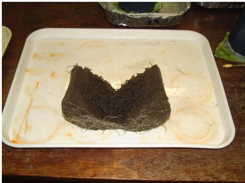
Figure 3 Soil core after the 2 month growing period (SSL; BD2). Roots generally explored the gaps between the cylinder and the soil with little root growth into the bulk soil.
