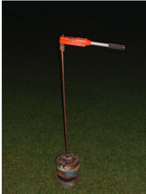
Figure 5 Traction test equipment. 41 kg of steel weights, plus the weight of the testing equipment equalled approx 45.5 kg. The studded plate is beneath the weights, in the turf.
