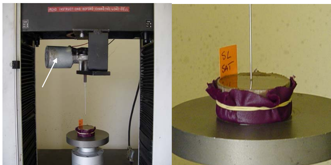
Figure 3.8 (left) A sample on the Instron loading machine. (Arrow indicates a motor to rotate the penetrometer which was not used during this study)
