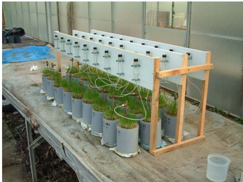
Figure 3.14 Tensiometers in each WG cylinder
