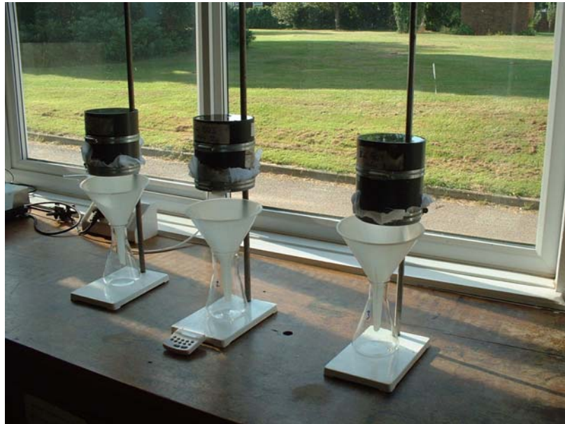
Figure 2 CL BD3 soil, saturated with a 50mm head of water. Note the absence of any drainage.
