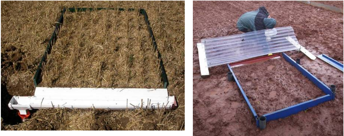
Figure 4.3-3 Micro-plot collection system (left) and protective covering (right)
