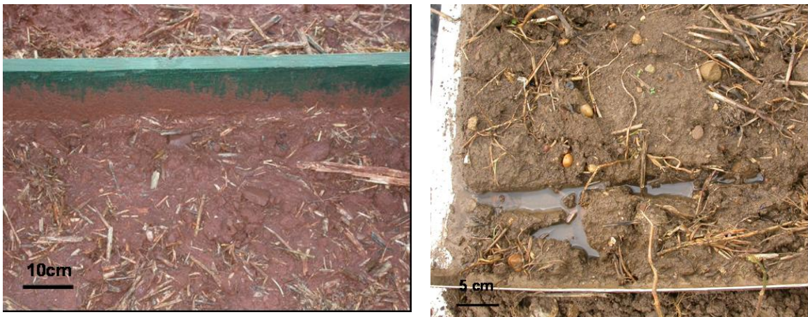
Plate 6.5-2 Splash erosion at Tivington (left) and overland flow at Loddington (right) during micro-plot trials
