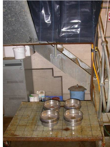
Plate 5.3-3 Rain tower apparatus; needle tray (top left), rainfall catch area (top right), and four sieves with saturated aggregates ready for testing (left)
