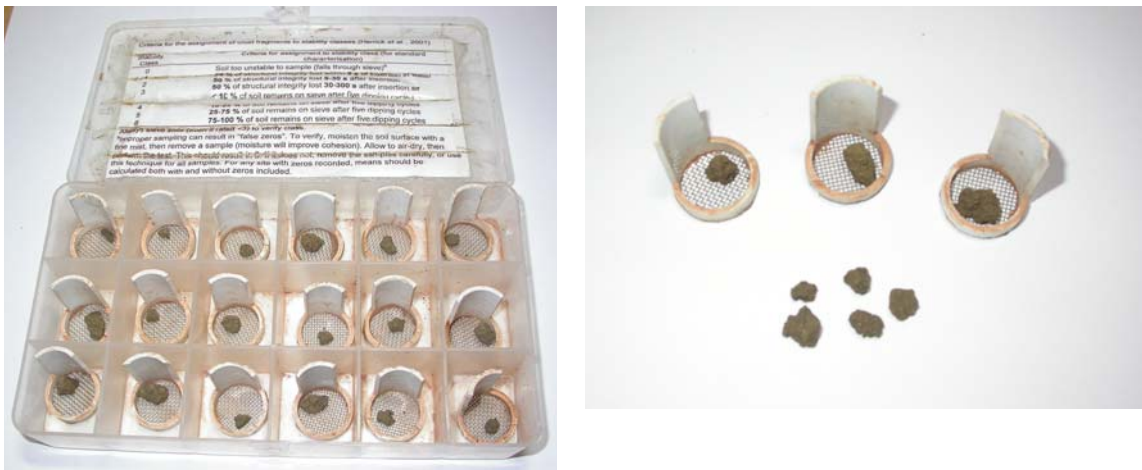
Plate 5.3-2 Field test kit (FTK) apparatus. Test box dimensions 21 x 10.5 x 3.5 cm. Sieve size 2cm diameter and 1.65cm aperture.
