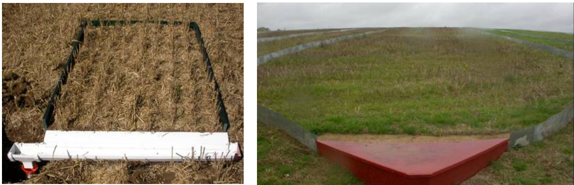
Plate 6.5-1 Micro-plot (left) width of 1m compared to field plot (right) plot width 9m (collection funnel 1.5m)
