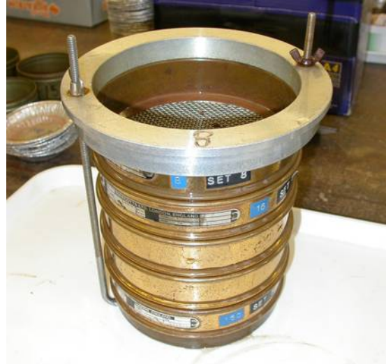
Plate 5.3-1 wet sieving apparatus (top left); a single stack of sieves (top right); retained aggregates after sieving (left)
