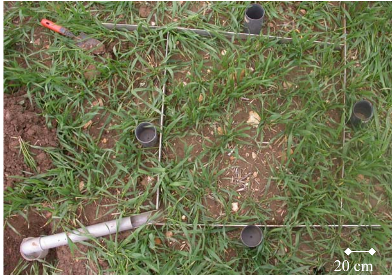
Figure 6.2: Photograph showing rainfall simulation bunded plot, rainfall catch cups and collection system.
