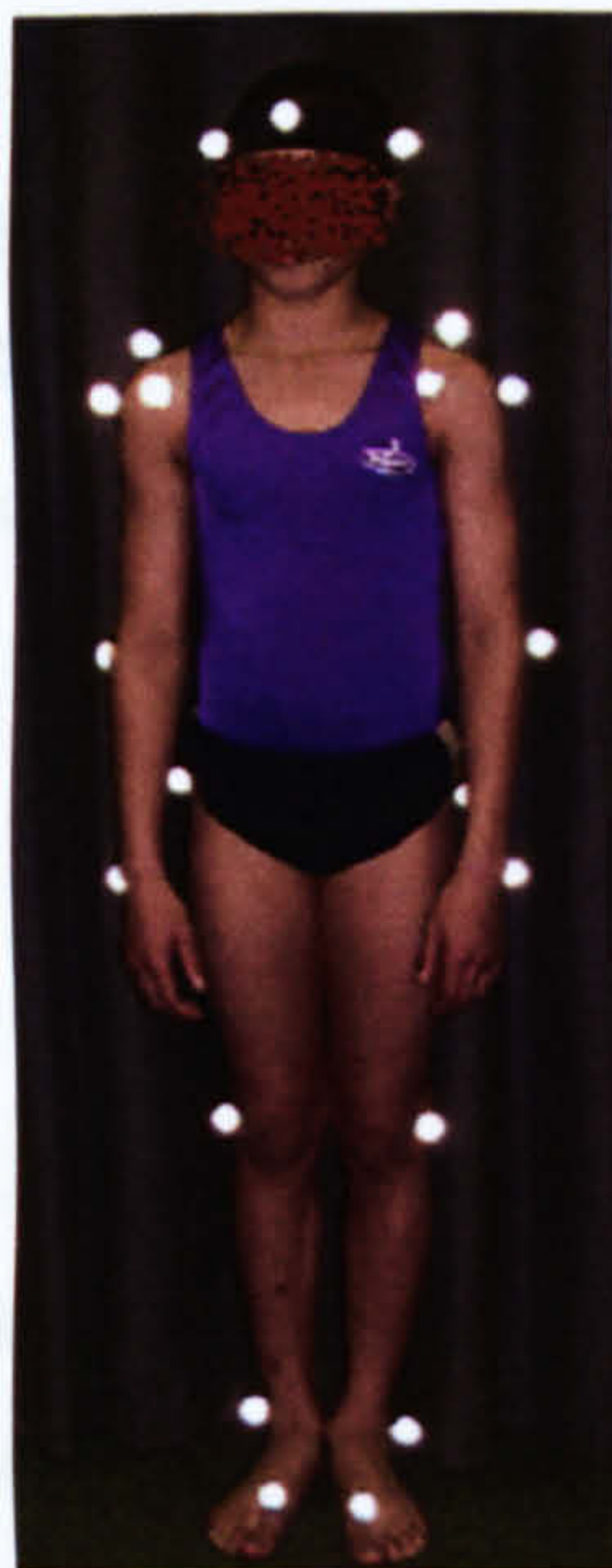
Figure 9-1: Marker placement for Vicon data collection.
