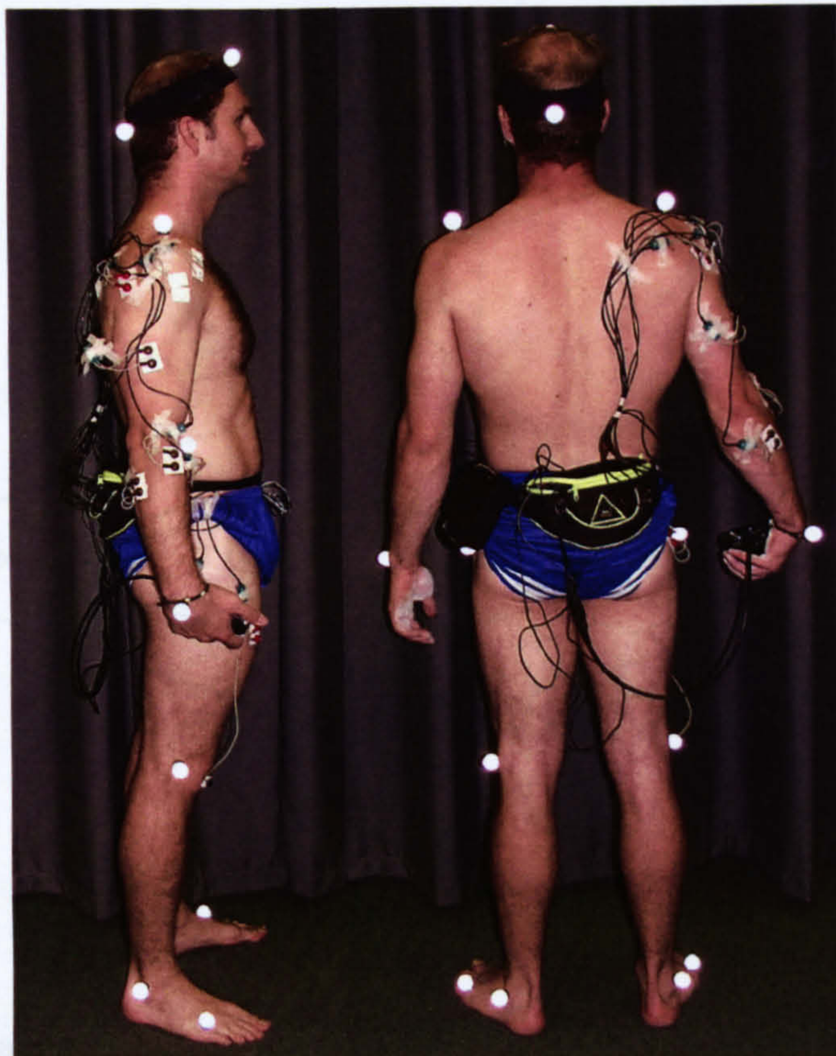
Figure 6-3: Gymnast R with EMG electrodes and Vicon markers.
