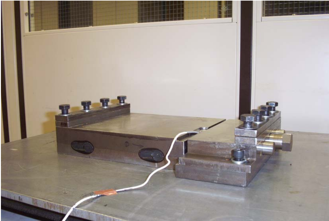
Figure B-4: Photograph of manufactured flat-bed prestress rig instrumented with load cell.
