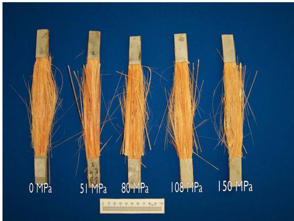
Figure 8-4: Photo macrograph of static tensile specimens.
