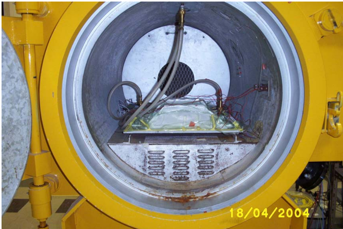
Figure B-5: Photograph of conventionally vacuum-bagged prepreg laminate clamped to the FBPM inside the autoclave.
