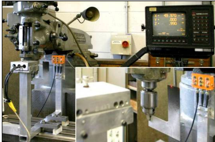
Figure 158: Alignment of diode lasers on milling machine bed
