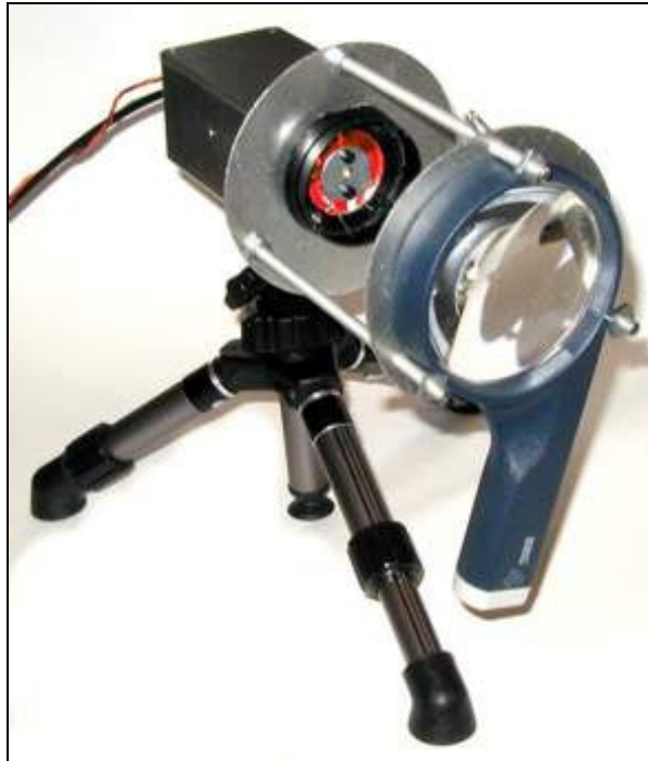
Figure 179: LED flash unit with Collimating Lens
