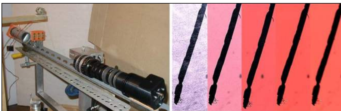
Figure 172: Test of LED flash unit and camera with resulting images at 100m/s.
