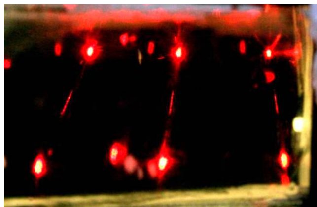
Figure 89: Laser beams intercepting the droplet stream and tunnel walls
