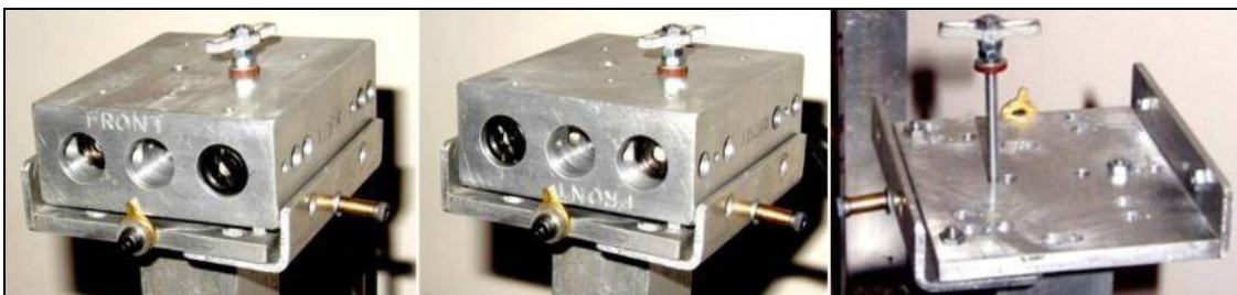
Figure 159: Arrangement for supporting and inverting the diode laser block.
