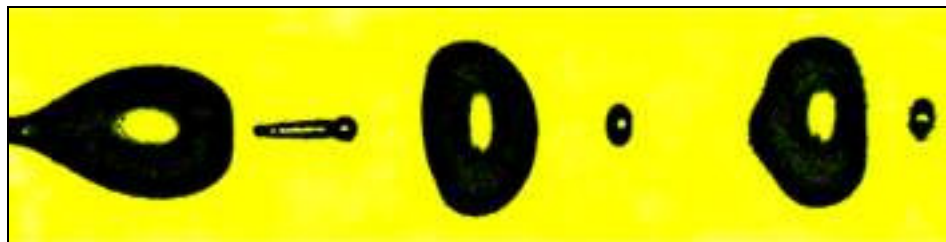
Figure 167: Droplet image obtained from strobe illumination with low-power LED
