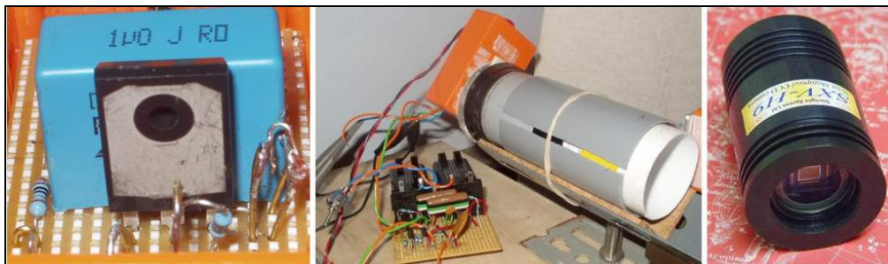
Figure 170: Prototype LED flash unit and Starlight Express astronomy camera
