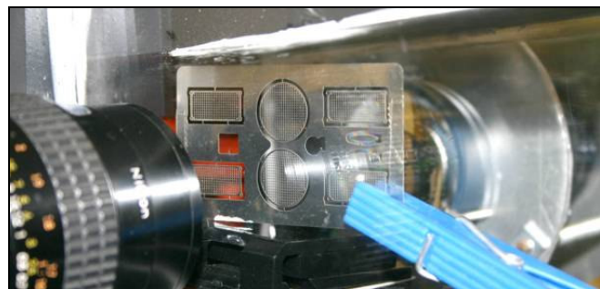
Figure 79: Using calibration grid inside the tunnel
