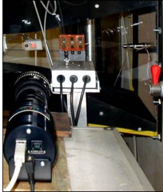
Figure 75: Wind tunnel test with prototype LED flash and Astronomy camera.
