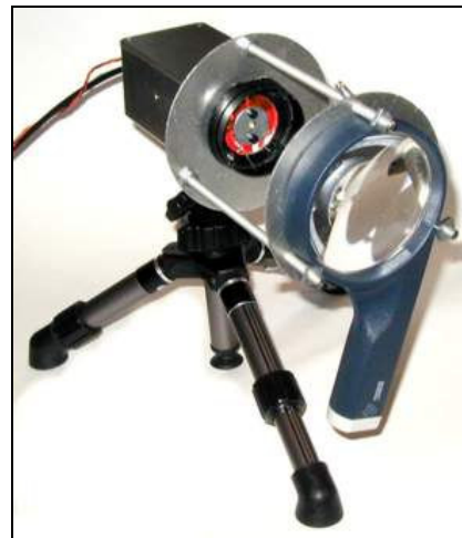
Figure 11: LED flash unit with 80\text{mm} Collimating Lens
