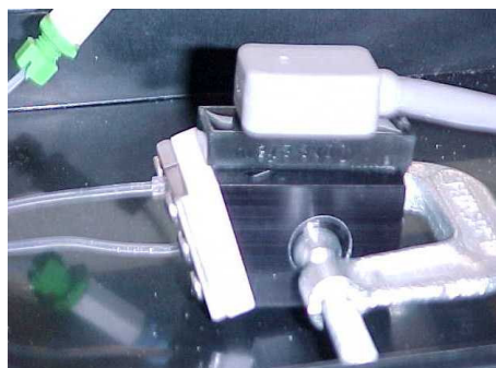
Figure 2.5: Photographic illustration of the original Spreeta™ G-clamp flow cell. The flow cell is connected to the SPR sensor by using a G-Clamp. The sensor is then connected to the control box via the connection lead. Fluid is introduced to the sensor surface via tubing of 0.25mm diameter.
