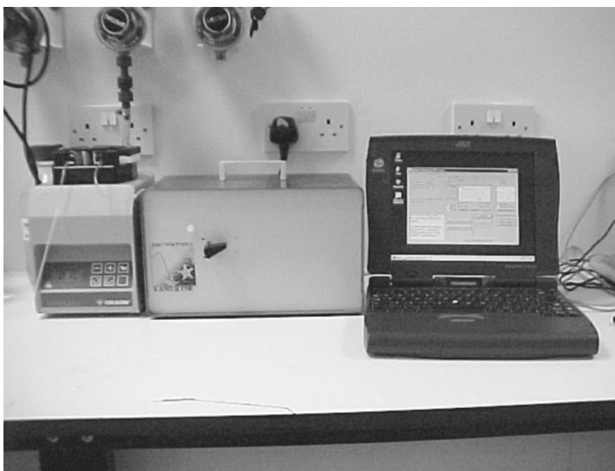
Figure 2a. External view of field-analyser showing external peristaltic pump and control notebook computer.
