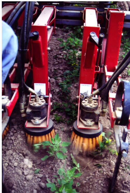
Figure 2-13 Vertical brush weeder
