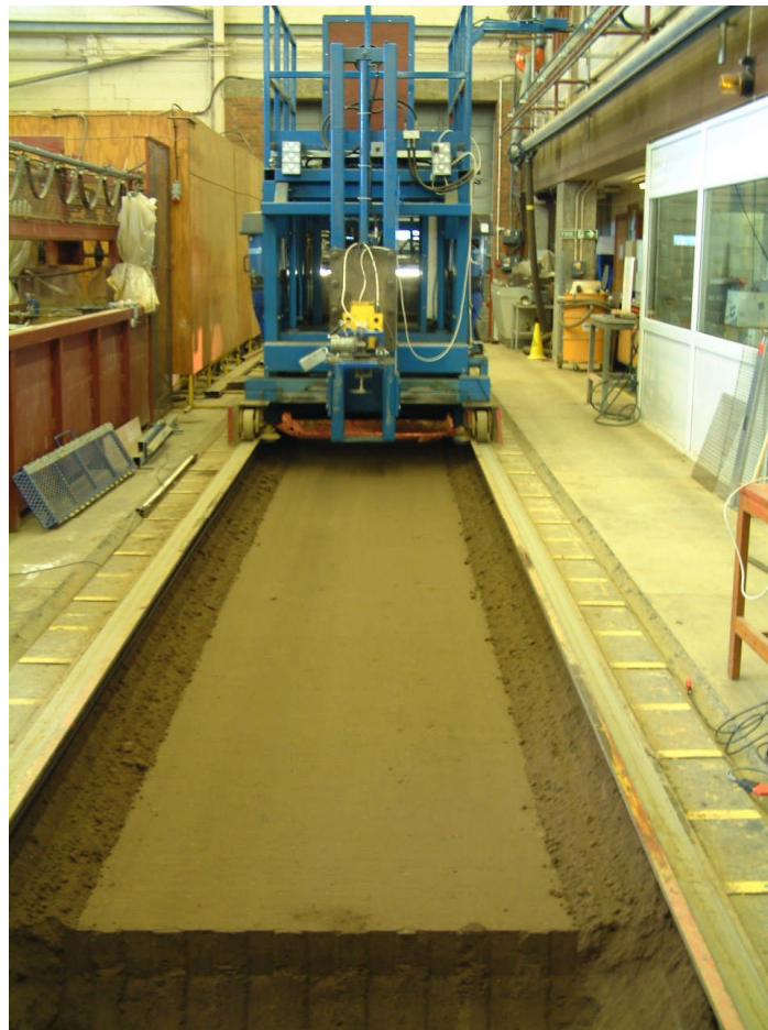
Figure 4-1 The soil bin and the processor
