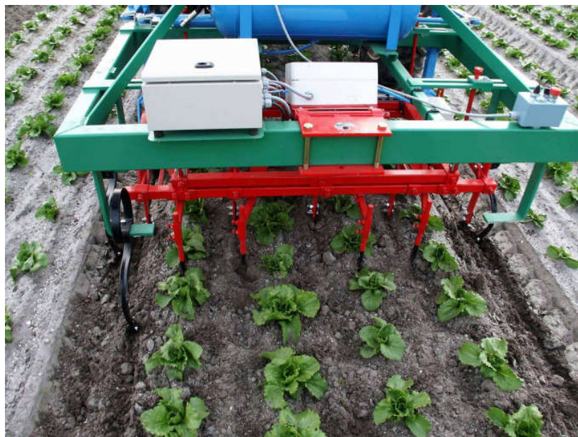
Figure 2-18 The Radis intra-row weeder (Bleeker, 2007)
