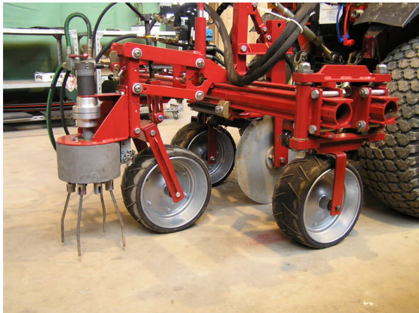
Figure 2-16 The cycloid hoe (Griepentrog, 2007)
