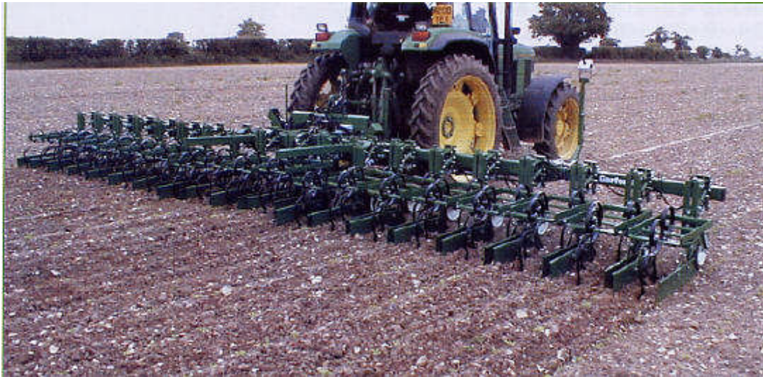
Figure 2-4 Tractor mounted hoe for inter row cultivation
