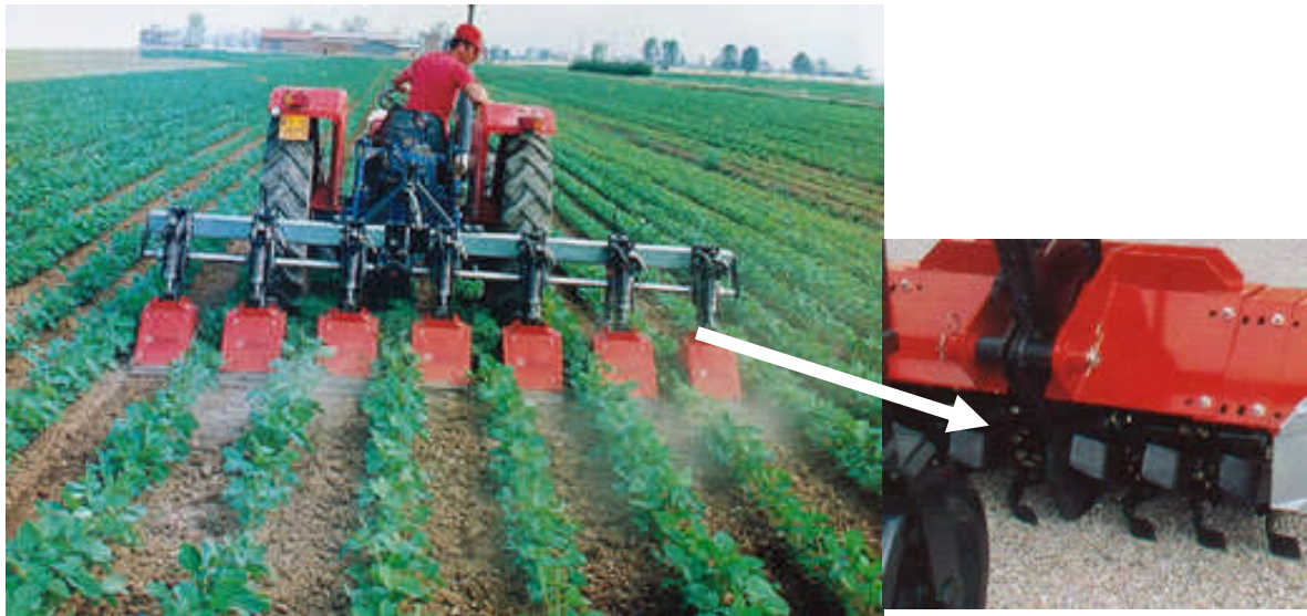
Figure 2-14 Powered rotary inter-row weeder
