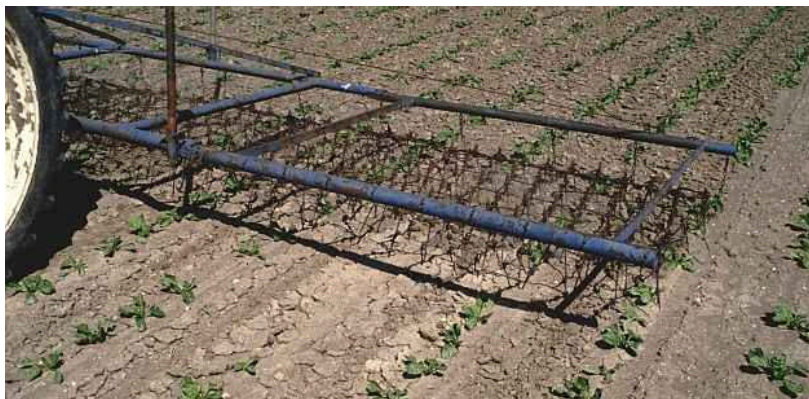
Figure 2-3 Flexible chain harrow weeder
