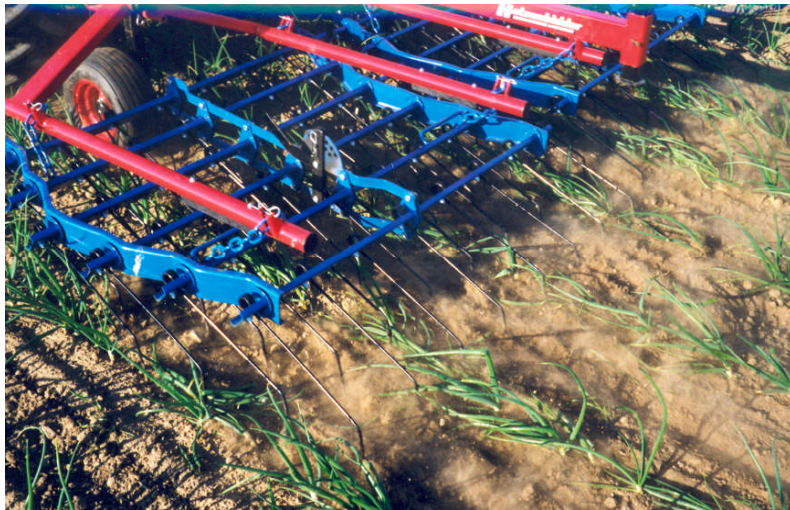
Figure 2-2 Spring-tine harrow weeder
