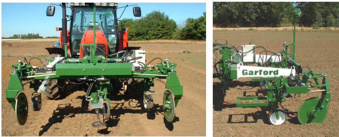
Figure 7-1 The prototype guided rotating disc hoe with one disc attached and a camera mounted 1.7 m from the soil surface
