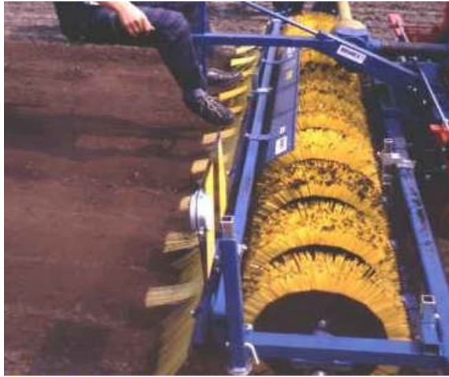
Figure 2-12 Horizontal brush weeder
