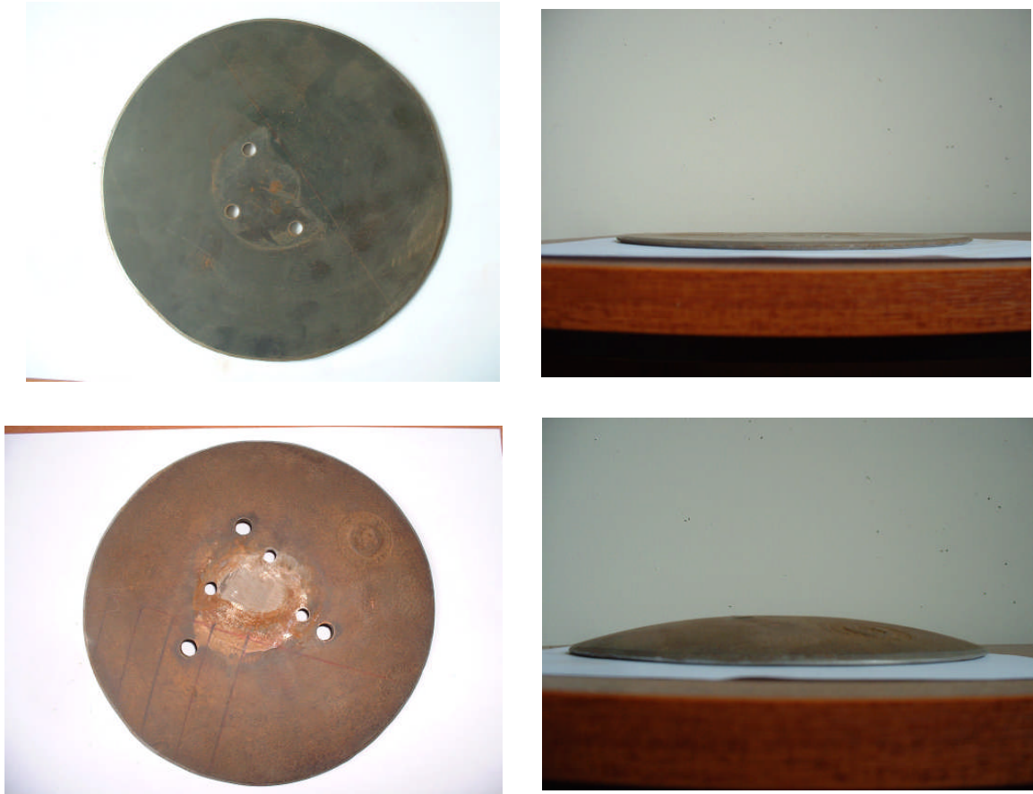
Figure 5-1 Disc geometries evaluated in the controlled laboratory experiments, flat (upper); convex (lower)
