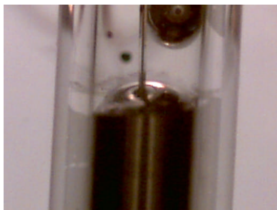
Figure 5.8: Platinum-quartz fibre-mercury junction in lumen of capillary
