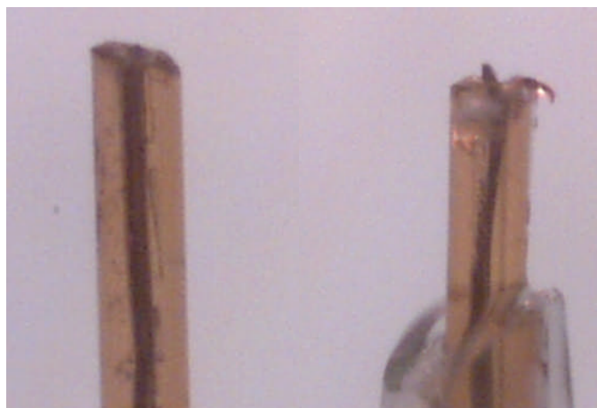
Figure 5.3: Optical Micrograph of 30 \mu m probe fabricated by Sycopel International
