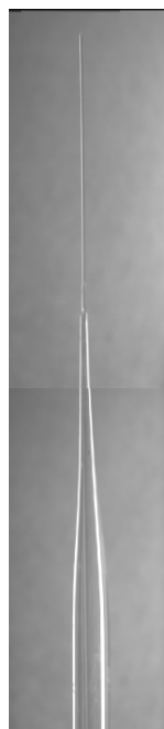
Figure 5.2: Optical micrograph of commercially available electrode from Thomas Recording GmbH
