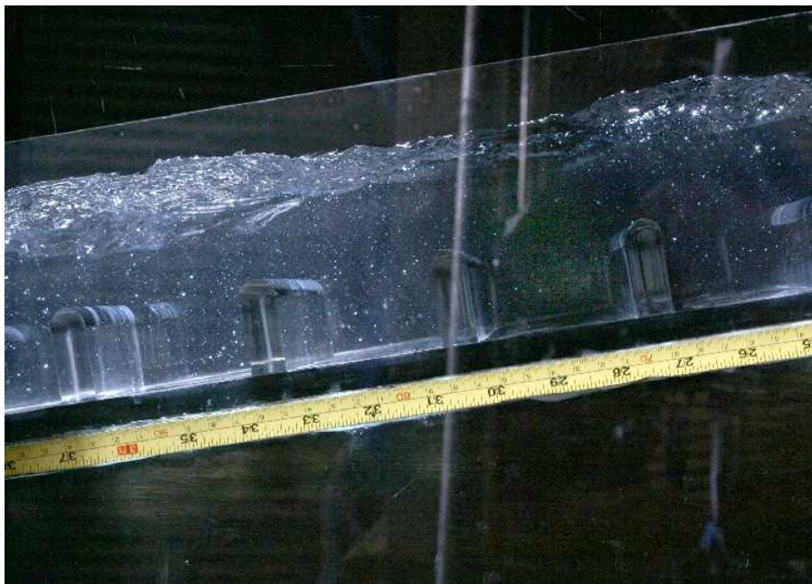
Figure 4–41: Free surface profile: unequal baffle pairing at the 10 percentile low-flow rate (baffles 8 to 12)
