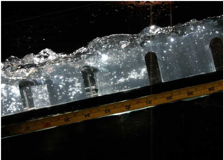
Figure 4-39: Free surface profile: unequal baffle pairing at the 50 percentile low-flow rate (baffles 8 to 12)
