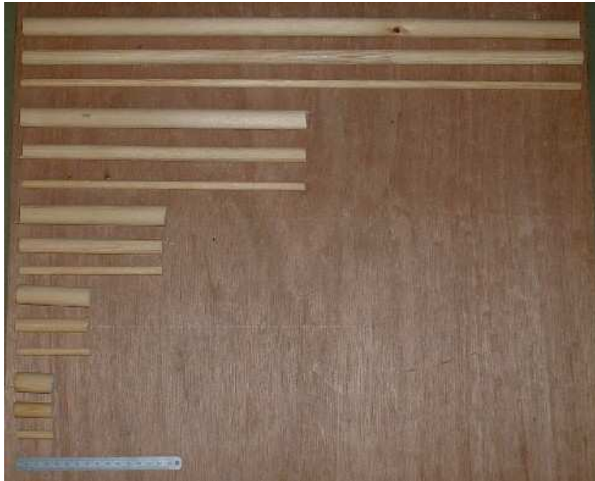
Figure 4–65: Debris: Photograph of the one of each length:diameter dowelling rod used
