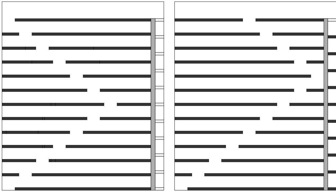
(a) Arrangement 2: LEGO layout 2.5 (Overlap = 16 mm), identical to Baffle layout 4) (b) Arrangement 4: LEGO layout 2.6 (Overlap = 16 mm)
