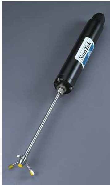
Figure 3–19: Sontek 16 MHz MicroADV
