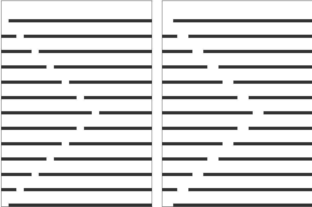
(a) Arrangement 1: Baffle layout 2 (Overlap = 32 mm, Slot width = 32 mm) (b) Arrangement 2: Baffle layout 4 (Overlap = 16 mm, Slot width = 48 mm)
