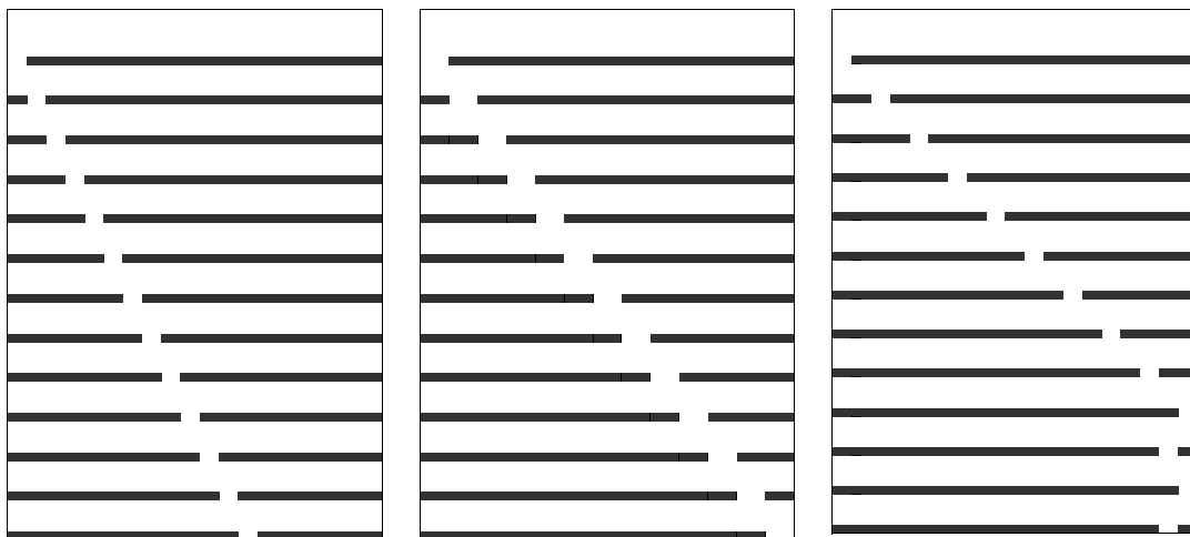
(a) Plan of Baffle layout 5 (Slot: 32 mm Overlap: 0 mm) (b) Plan of LEGO layout 1.1 (Slot: 48 mm Overlap: 0 mm) (c) Plan of Baffle layout 6 (Slot: 32 mm Overlap: 32 mm)
