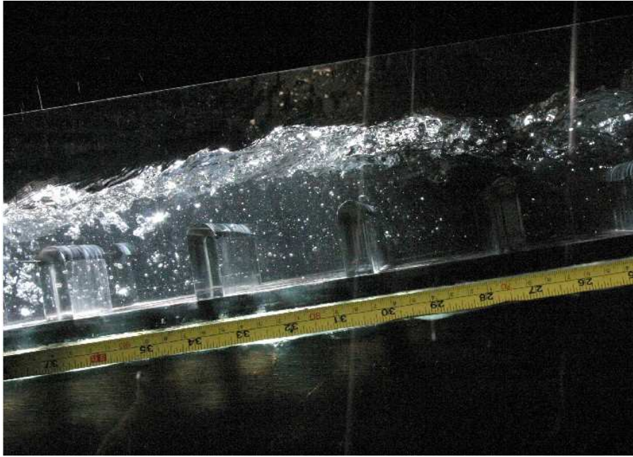
Figure 4–40: Free surface profile: unequal baffle pairing at the 30 percentile low-flow rate (baffles 8 to 12)
