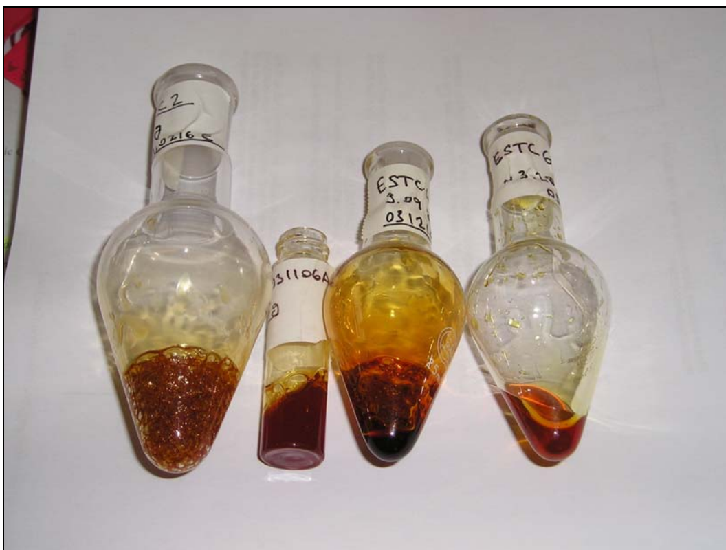
Figure 2.13 A picture of Polymers (from left to right): 1 (ES%=76), 2 (ES% =70), 3 (ES%=61%) and 5 (ES%=51), showing apparent trend of decreasing viscosity.
