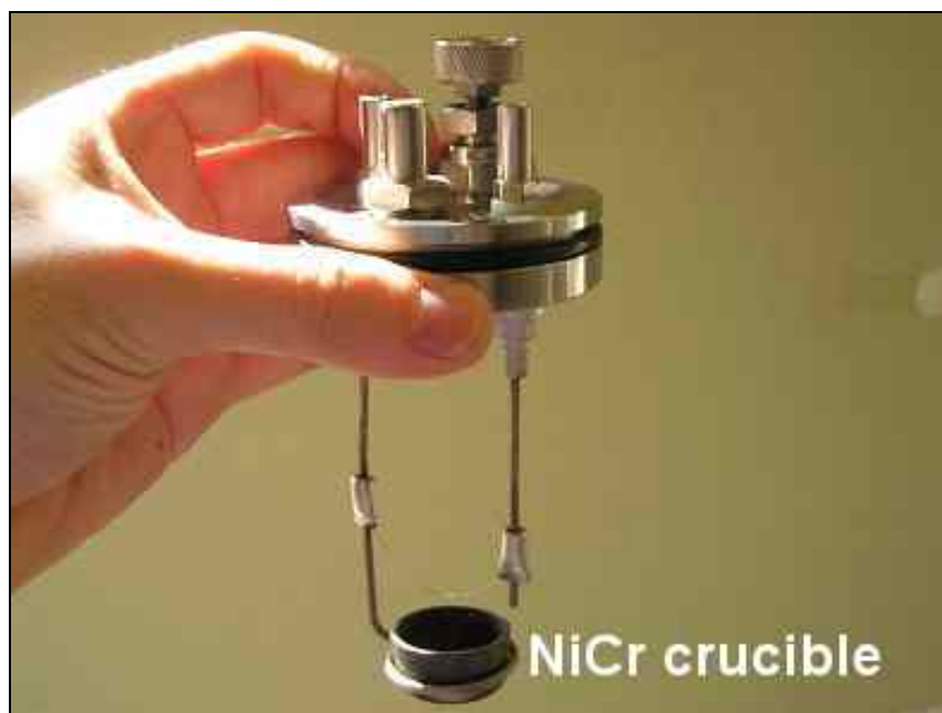
Figure 2.18 Parr 1108-Cl bomb twin-valve lid with crucible in place
