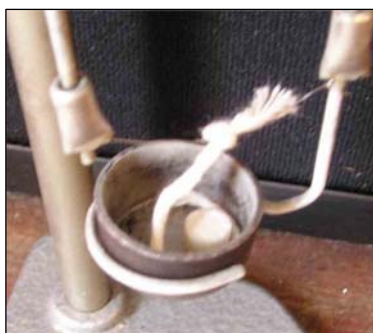
Figure 2.55 Alumina crucible loaded with linear poly[bis(2,2,2-trifluoroethoxy)phosphazene] inside the main bomb crucible, ready for combustion.
