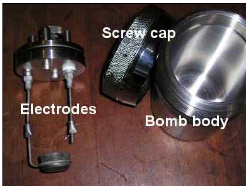
Figure 2.17 Parr 1108-Cl bomb's three main components
