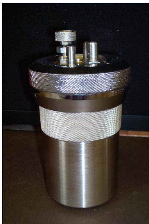
Figure 2.16 The Parr 1108-C1 twin-valve, halogen-resistant ‘Hastelloy’ bomb
