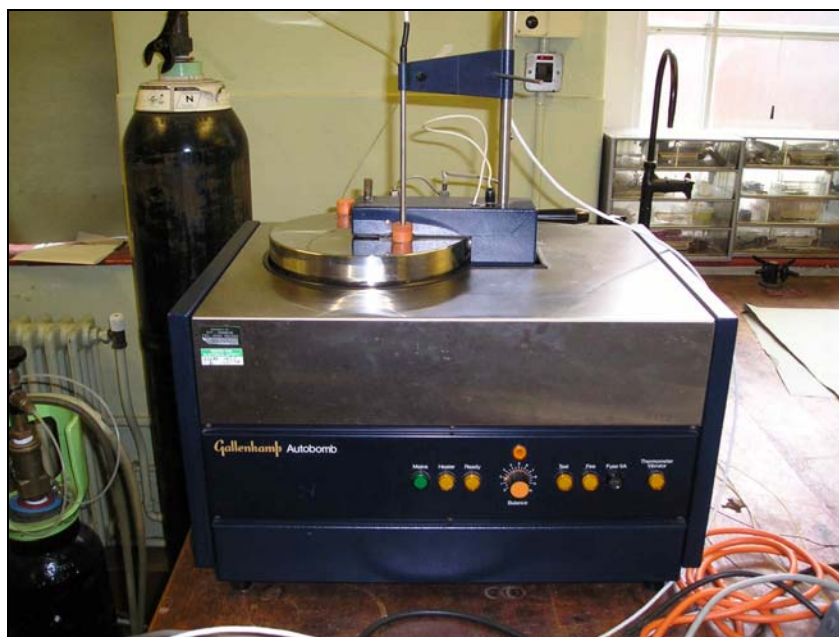
Figure 2.14 The Gallenkamp 305 ‘Autobomb’ static adiabatic calorimeter
