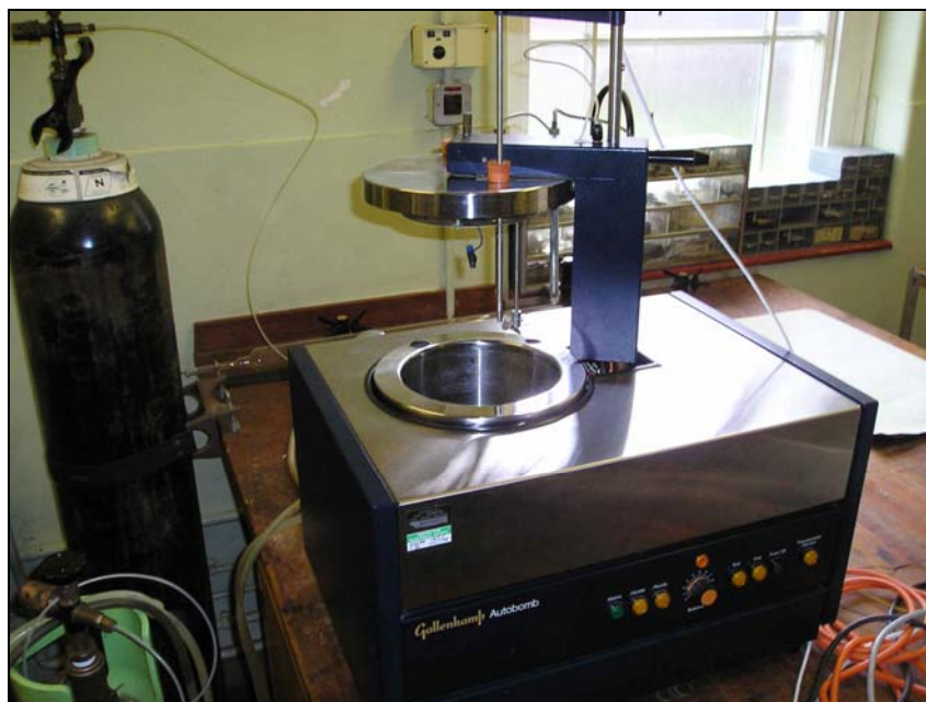
Figure 2.15 The Gallenkamp 305 ‘Autobomb’ static adiabatic calorimeter with jacket lid raised.
