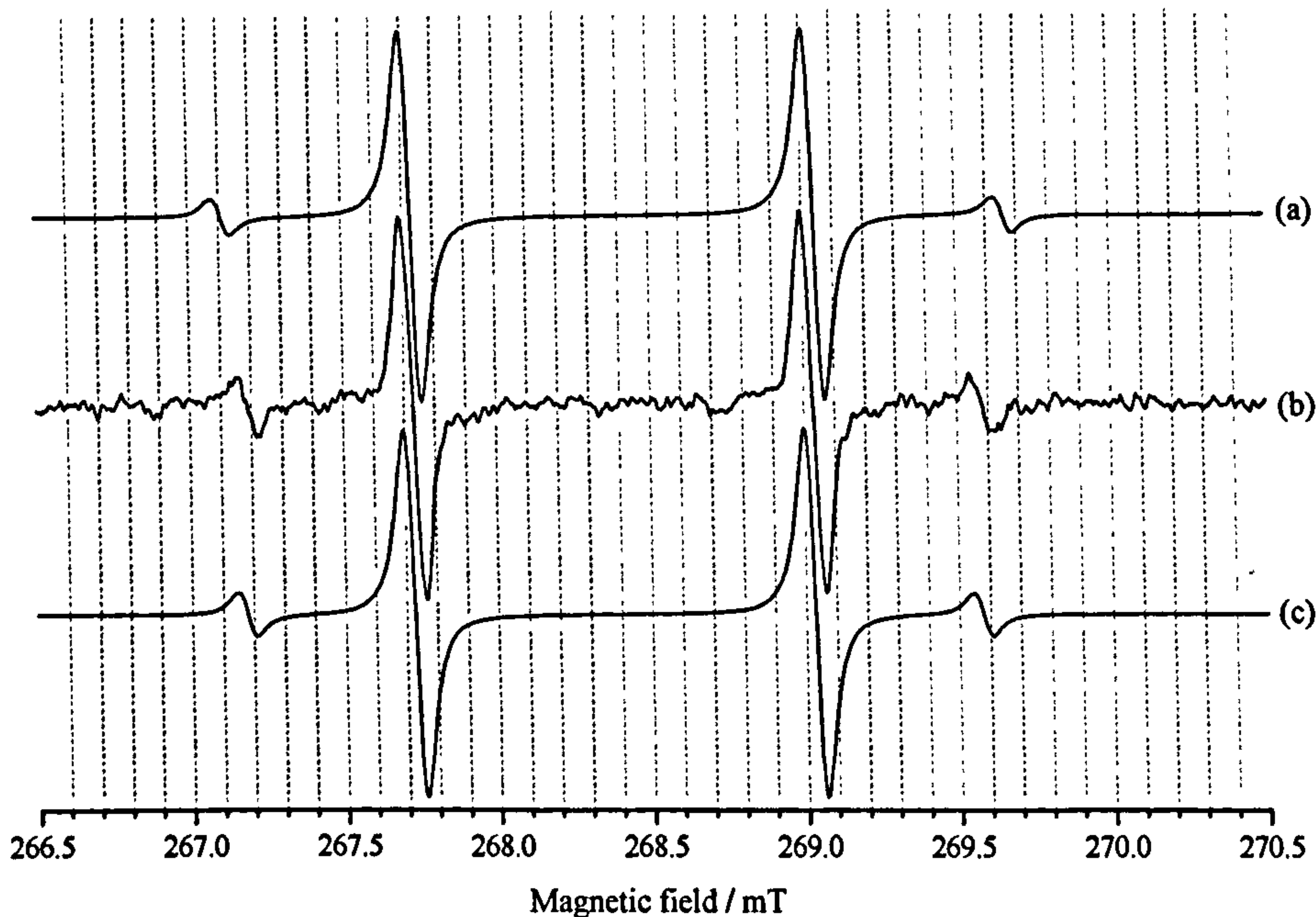
Figure 8-11: Lowest field pair of lines from the S = \frac{3}{2} defect observed with the applied magnetic field along \langle 111 \rangle . The weak, outmost lines originate from forbidden electron-nuclear double-spin flips. (a) shows simulated data assuming positive values for A_{\parallel} and A_{\perp} (b) is the experimental data and (c) is simulation obtained using negative values for A_{\parallel} and A_{\perp} . D > 0 for both simulations.
