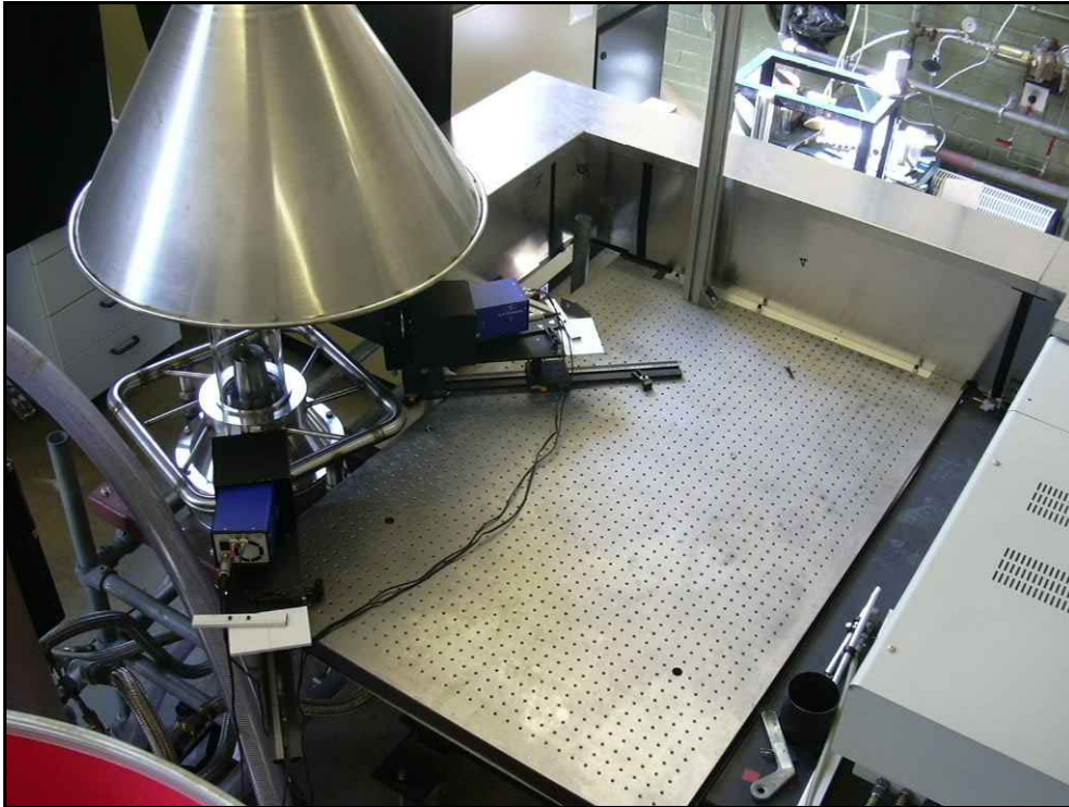
Figure 5.2. Stereoscopic PIV experimental apparatus used in Test House 1 at Cranfield University.
