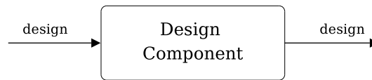
Figure 1.2: A design component accepts a design and produces a new design. Input and output may be routed to other design components.
