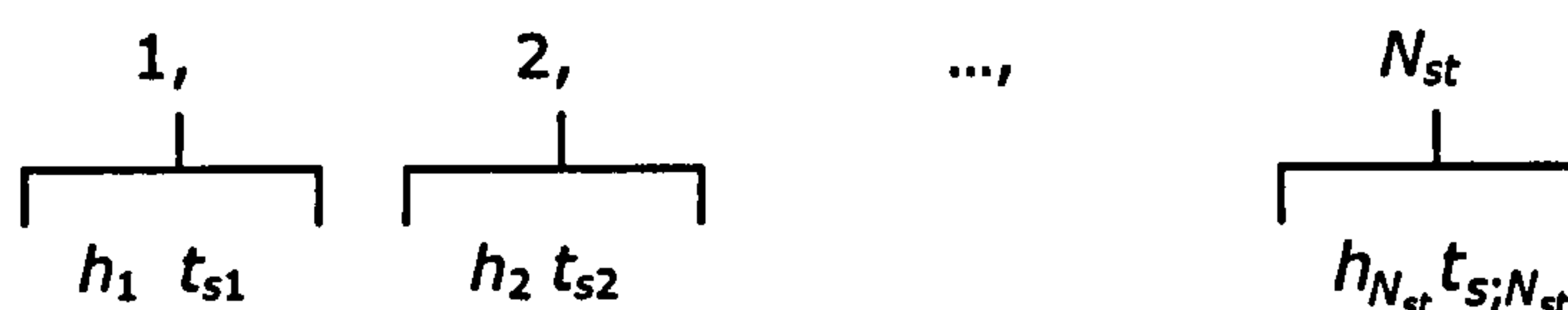
Figure 7.11 A sequence of storms and the pairs of water level and storm duration that represent each storm
