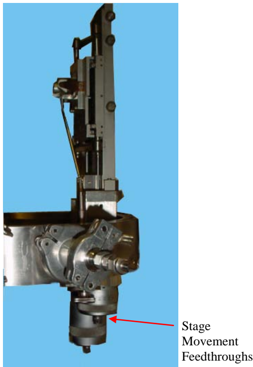
Figure 5.3: Image to show micrometer feedthroughs of sample stage on the HPVA
