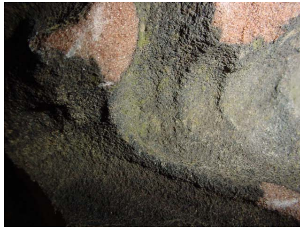
Figure 6.70: Image of weathered sandstone sample, showing green algae build-up
