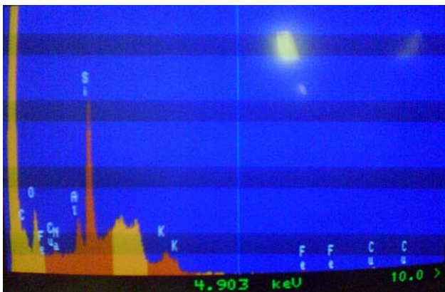
Figure 6.37: Sandstone EDX image
