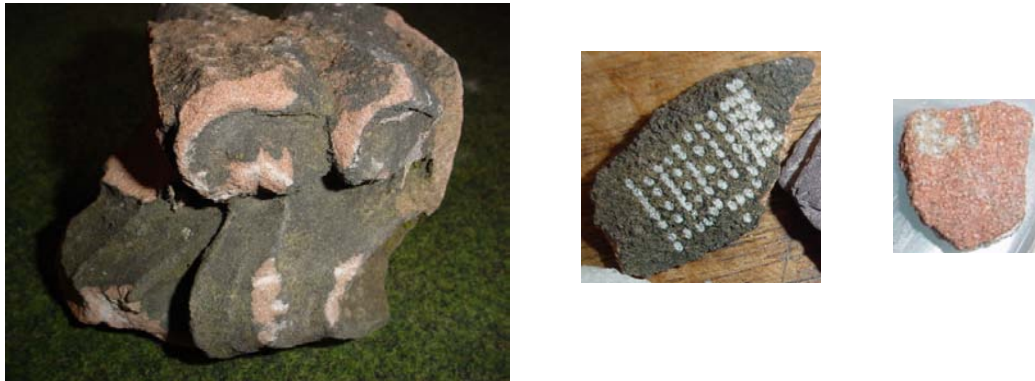
Figure 6.26: Images of sandstone samples, with ablation craters clearly visible. Both were taken from a larger block shown on the left, where organic residues can be seen building up on the surface, the clean stone visible underneath.
