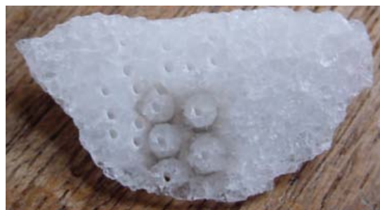
Figure 6.33: Images of marble samples, the one on the left showing the crystalline structure, the one on the right showing the ablation craters and in some cases the re-deposition from a partial or full methane content atmosphere.
