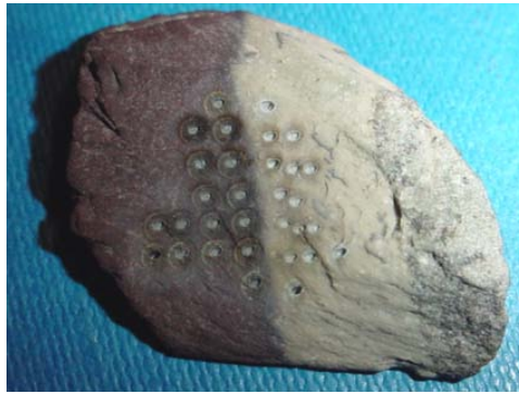
Figure 6.28: Slate sample showing ablation craters and re-deposition of material around the crater.
